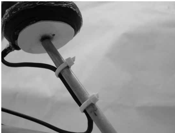
Figure A.7: GPS detail, silicone sealed connection between mast and nail
