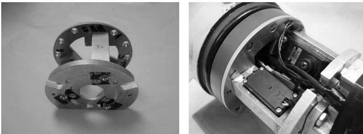
Figure 2.4: Set of brackets to which electronics mount; their mounting to tail
