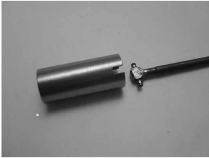
Figure 2.3: Dogbone shown next to slots into which it mounts on motor coupler
