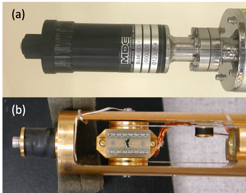
Figure 2.16: (a) The linear manipulator that controls the rotation of the sample holder to achieve various magnetic field orientations relative to the film plane.(b) The Janis tilting probe sample holder, by tilting which both parallel and perpendicular magnetic field can be achieved.
