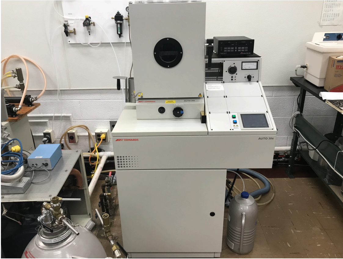
Figure 2.13: The thermal evaporator used to deposit Au film Ohmic contacts.
