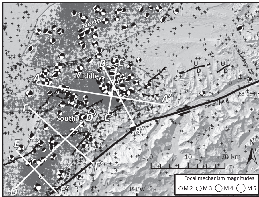
Fig. 11. Shallow crustal seismicity patterns near the Mount McKinley restraining bend. Previous studies divide the seismicity of the Kantishna cluster into north, middle, and south zones (Burris, 2007; Ruppert et al., 2008). Background seismicity is notably sparse to the east of the eastern vertex, along the trace of the Denali fault, and south of the Denali fault. Seismicity shown for 1968–2013 with depths of <25 km, although most hypocenters occur at <15 km depth. Focal mechanisms for this time period exhibit predominantly reverse and strike-slip displacements. White lines show the section lines for the seismicity cross-sections in Figs. 12 and 13.
