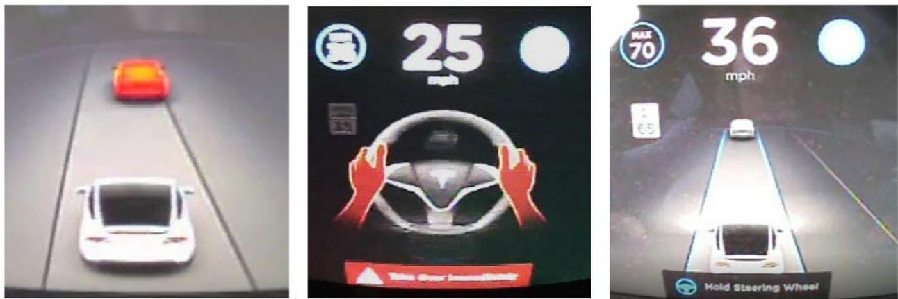
**Figure 1. Example of FCW, Immediate Takeover, and Hands-on-Wheel alerts in the VCC L2 NDS (Dunn et al., 2019).**
