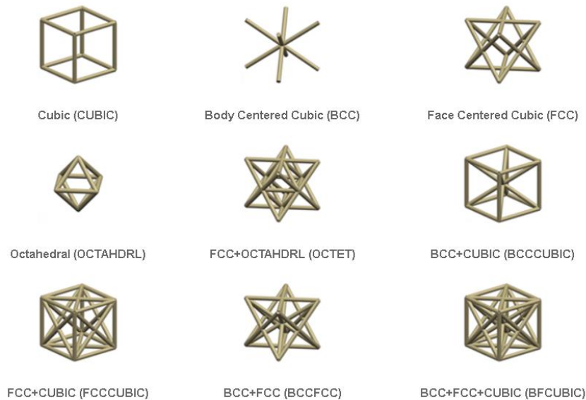
Figure 1-3. Lattice material interpolation methods allow for a third state in the topology optimization (solid, void, and lattice) are available in Simcenter Nastran 2019.2 [7][8].
