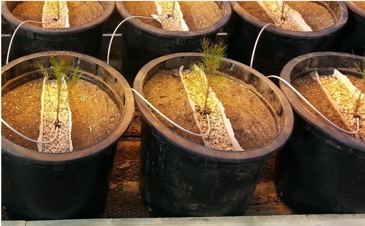
Figure 4.1. Each pot was filled with a pea-gravel base, a central dividing region of same gravel, and two distinct soil zones, see Methods for further details (Picture taken on 02/02/2016, three weeks prior to the switch to two drippers per pot)
