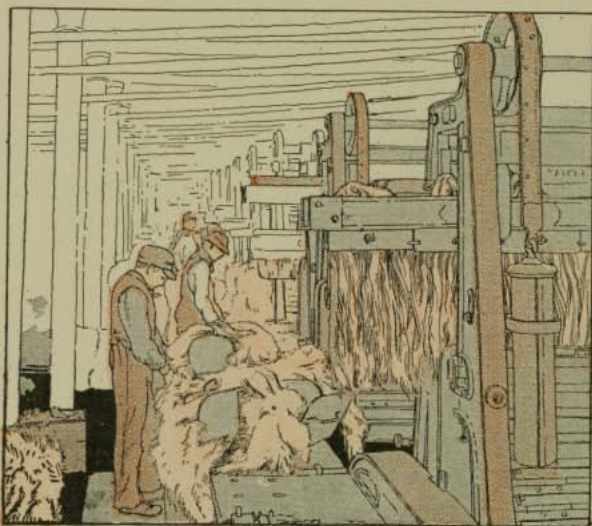
FIG. 177. — Flax hackling by machine.
