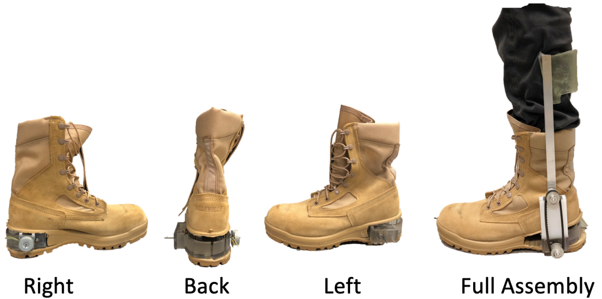
Figure 3.5- Right back and left views from boot harvester excluding timing belt assembly, and full assembly of the energy harvester.
