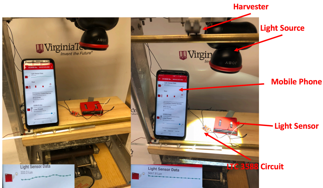
Figure 5.11- Power generated from the harvester is used to power the sensor and send a signal to a mobile phone to measure luminosity.
