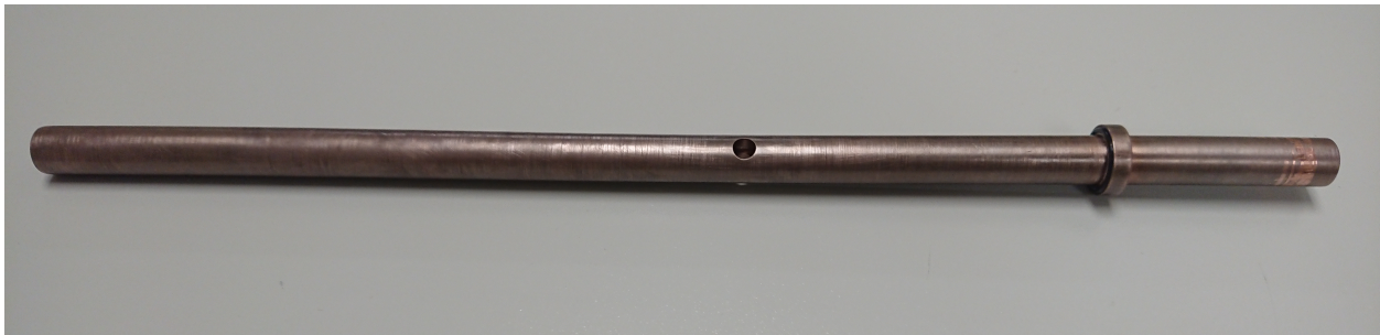
Figure 3.5: Photograph of the inner electrode. Note the holes approximately halfway along the electrode where the injected gas from the puff-valve is released into the breech of the gun. Also note the step near the right end where an o-ring forms a seal against the internal insulator. A region of lighter coloration at the far right end indicates the location of the inner power feedthrough collar.
