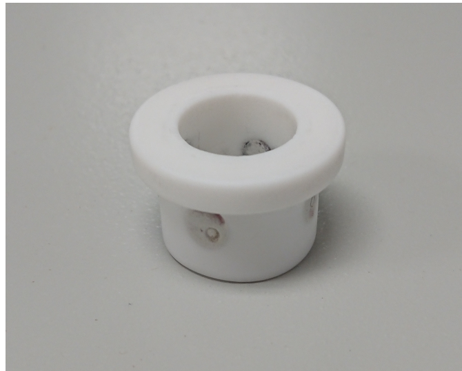
Figure 3.6: Photograph of the plasma-facing insulator. The breech surface is facing upwards in this photograph.
