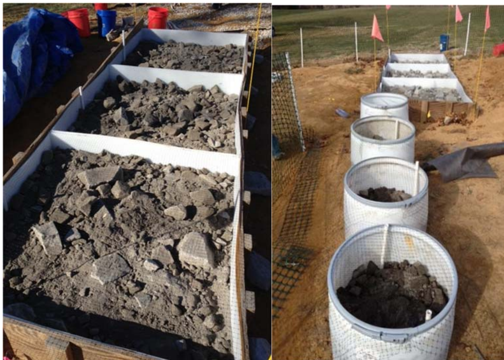
Figure 9. Harlan spoil leaching mesocosms (left) and barrels (right foreground) at Virginia Tech Turfgrass Research Center (VTRC) in November 2012. Leachates were collected monthly or following significant precipitation events and analyzed for pH and specific conductance. Ion composition was also monitored periodically (not reported here).
