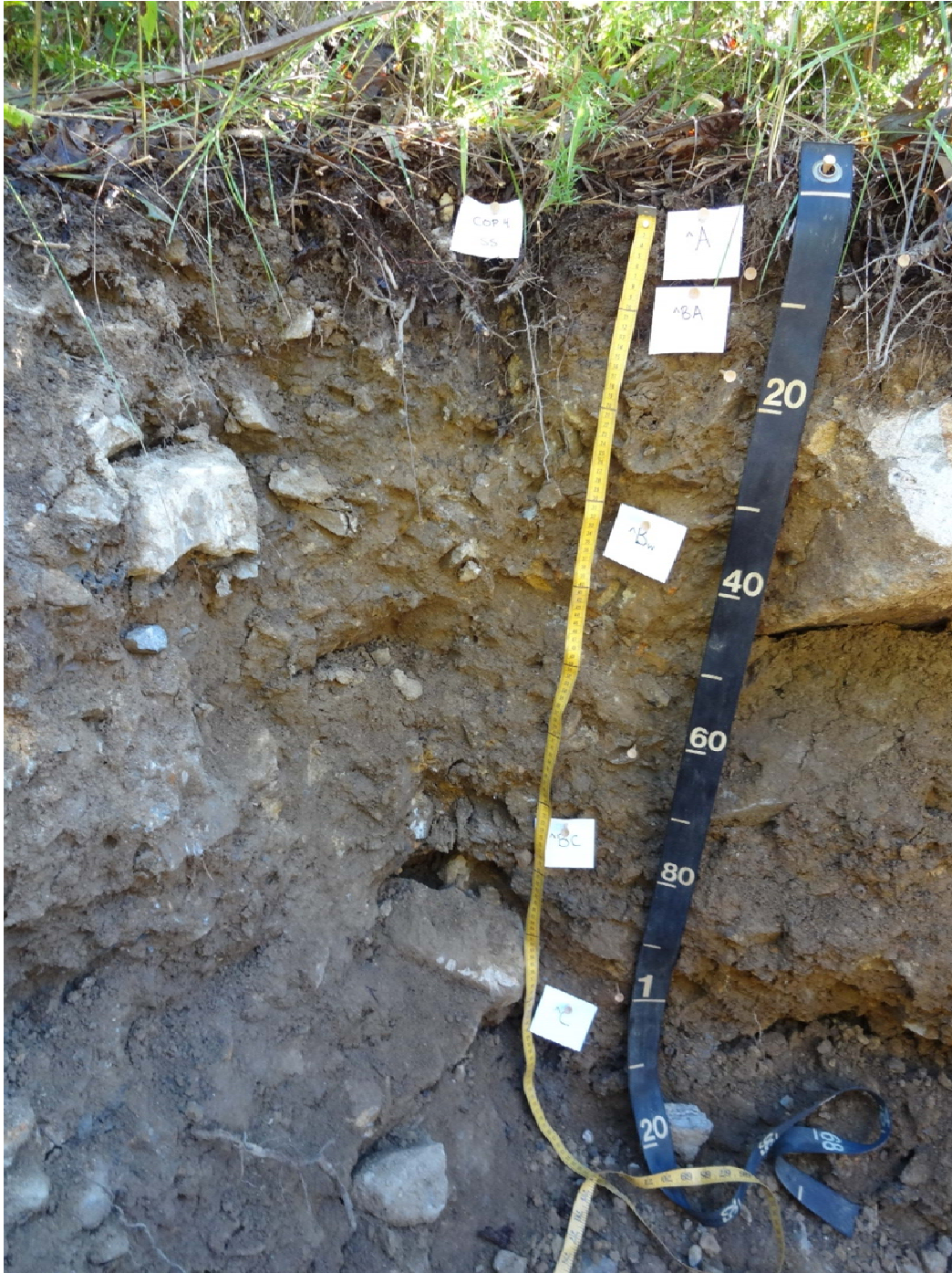
Figure 2. Soil profile described in 100% sandstone derived mine soil in plot #4. Note the relatively loose nature of the deeper C horizon material with open “bridging voids” along with the linear void below the large gray unweathered rock fragment on the upper right. However, the ^Bw horizon was quite compact relative to original conditions described in the same treatment in the 1980’s. The original sandstone spoils that were used were comprised of approximately 2/3 slightly pre-weathered “brown” sandstone and 1/3 hard gray non-weathered rocks that are so prominent in this profile.
