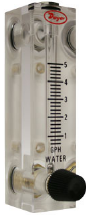
Figure 3.3: Dywer water flow meter. The flow meter has a working range 1-20 GPH and accuracy of 3% full scale
