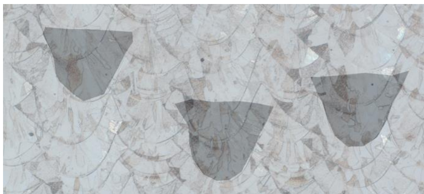
Figure 2.12 Overlay image of melt pool tracing on the optical image to determine average melt pool characteristics.
