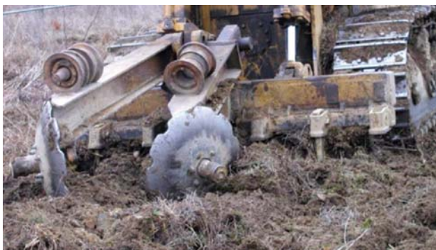
Photo 6. Coulters wheels on the back of a dozer, with ripping tooth inserted into the soil. The coulters wheels pile loosened soil into a mound, allowing seedlings to be planted at a slightly elevated position above the land surface. Use of coulters wheels is advised for mine soils with poor water drainage and few large rocks.
