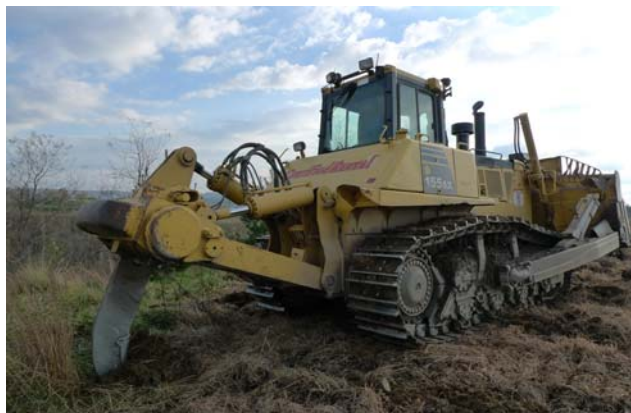
Photo 4. The ripping tooth on the back end of this dozer can be inserted into and pulled through the ground to loosen the dense mine soil, improving its physical properties and ability to support planted trees.
