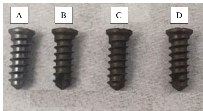
Figure 4: A: Untreated Ti-6Al-4V alloy screws (Control A). B: APTES-DA treated screw (Control B). C: GO coated screw (Group 1). D: C-GO coated screw (Group 2)
