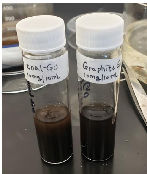
Figure 2: c-GO and GO suspensions used for coating
