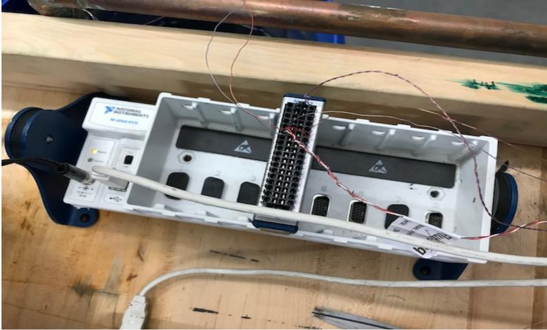
Fig. 25 NI9213 Data Acquisition with the thermocouples and the heat flux wires.
