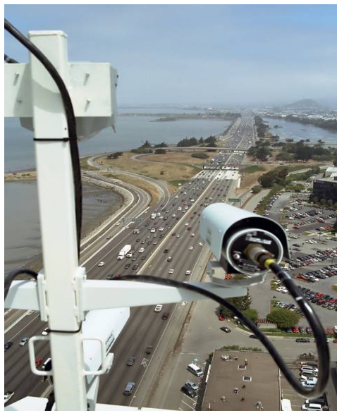
Figure 4-1. A digital video camera mounted on top of a building that overlooks a highway is recording vehicle trajectory data.
