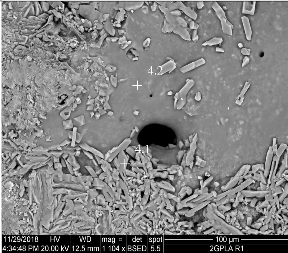
Figure 2.5 Granulated poultry litter ash (GPLA) backscatter electron dispersive (BSED) elemental analysis of multipoint identified structures (Pts. 4.1 and 4.2).
