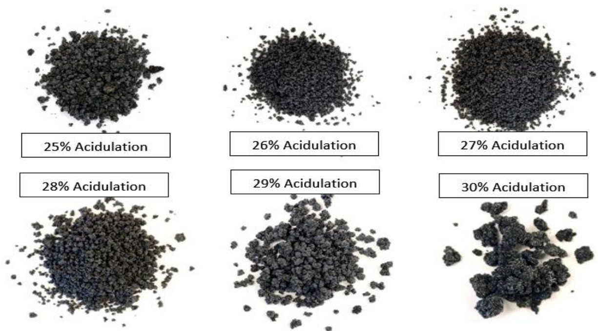
Figure 3.6 Granulated Poultry Litter Ash acidulation trial 2 (GPLA-Acd2) visual effect on granule size.
