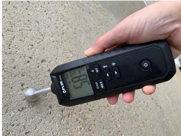
Figure 6.9: The FlirTM MR59 moisture meter used in this work. To take measurements, the end of the sensor is placed against the wall and held in place.
