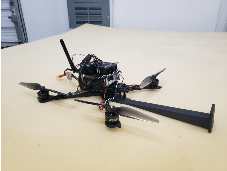
Figure 6.15: Prototype UAVs for testing path planning and control algorithms for contact-based inspection.
