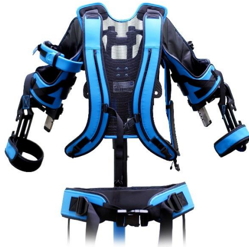
Figure 1. 2 EksoUE is a wearable, upper-extremity exoskeleton designed to assist a patient's affected shoulder and arm during rehabilitation. Image downloaded from https://eksobionics.com/eksoue/
