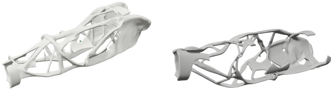
Figure 2. 9 Generative design model examples without outer boundary limit
