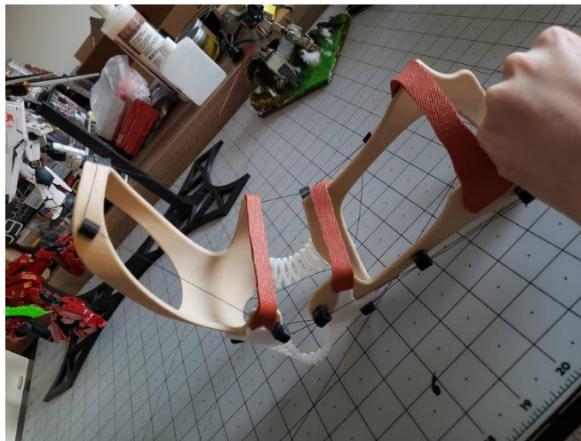
Figure 3. 19 Prototype 2.0 cable articulation test
