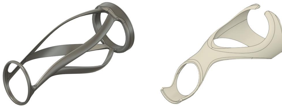
Figure 2. 4 Traditional CAD design of forearm exoskeleton frame
