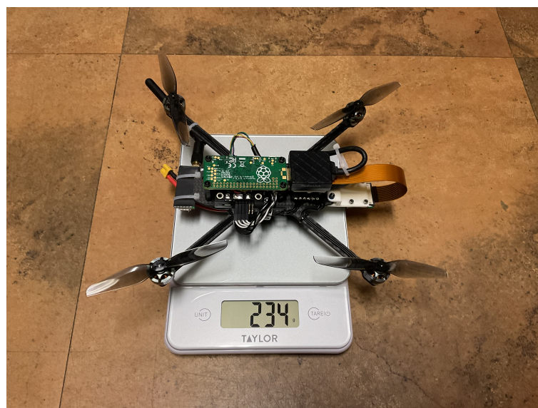
Figure 4. Our small, low-cost drone which weighs under 250 grams.
