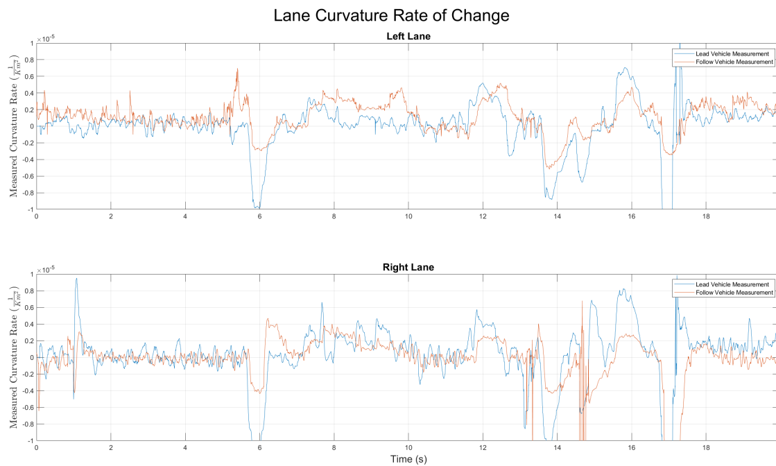
Figure 2.6: Headway adjusted curvature rate of change parameter raw values. The lead and follow vehicle lane parameters are aligned for comparison.
