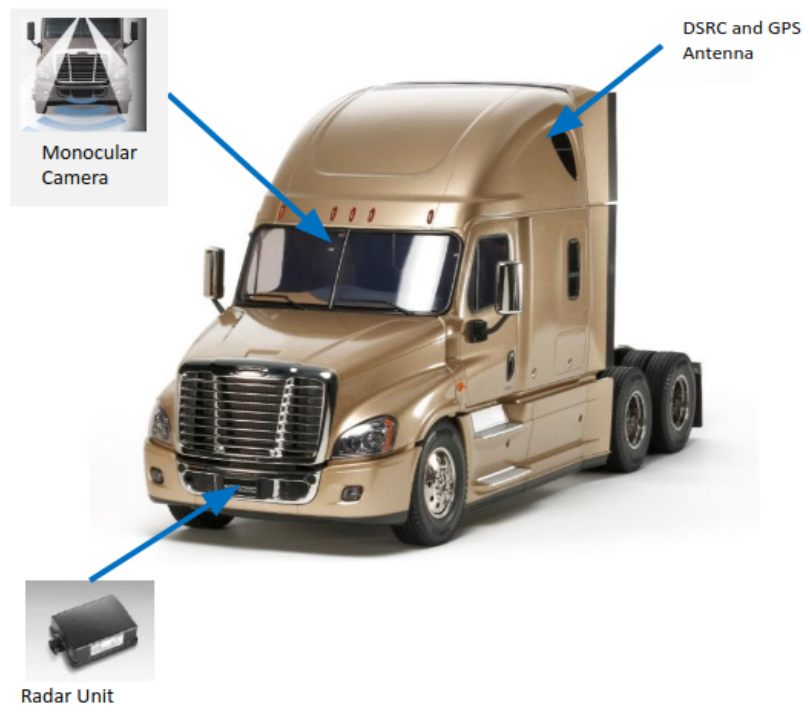
Figure 2.2: ADAS set implemented on DTNA Truck Pairing Program prototype vehicles https://freightliner.com/
