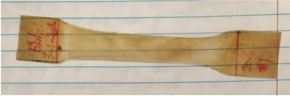
**Figure D.6.** Uniaxially stretched dogbone
