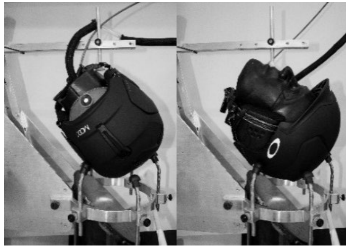
Figure 1.1: Snowsports helmets were tested at two impact locations, rear boss (left) and side (right). Helmets were dropped onto an oblique anvil of 45° under two friction conditions (low and high).
