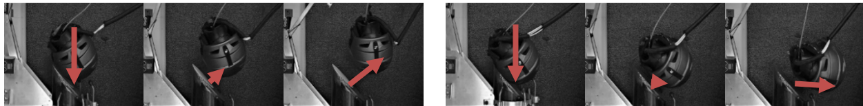
Figure 1.4: High speed video frames of two exemplar side impacts. The low friction condition (right) reduced PLA because the helmet slid down the anvil, causing a lower velocity change.
