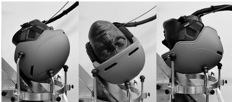
Figure 3.1: Snowsports helmets were tested at three impact locations, rear boss (left), side (middle), and front (right). Helmets were dropped once at each of these positions onto an oblique anvil of 35° and 55°.
