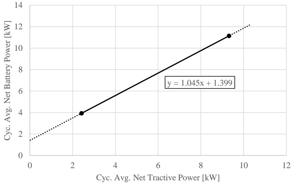
**Figure A.8:** 2021 Mustang Mach-E Extended Range EPA Net Willans Line
