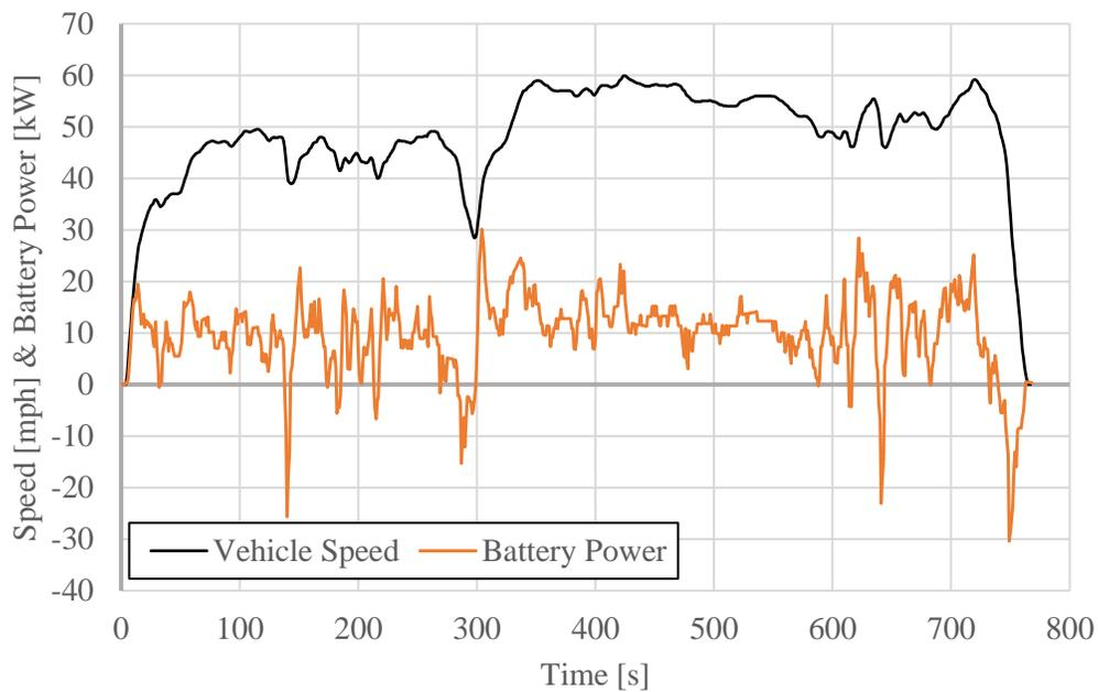
**Figure 3.7:** Highway Drive Cycle Speed Profile and Battery Power
