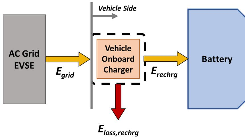
*Figure 3.5: Vehicle Recharge Power Flow*
