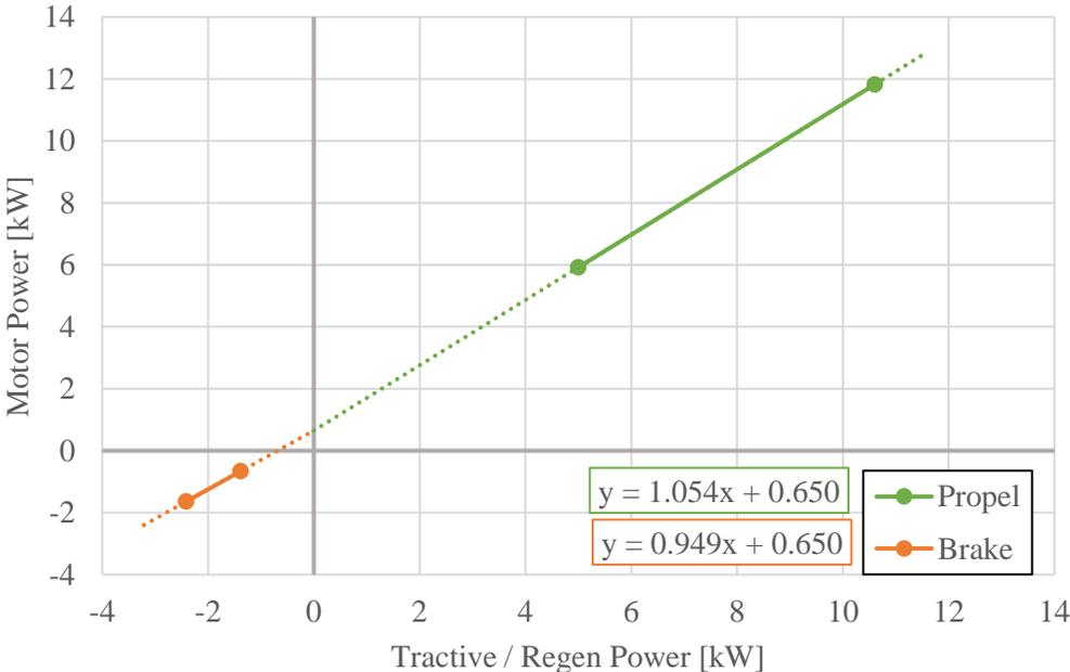
**Figure A.5:** 2021 Mustang Mach-E Standard Range Bi-Directional Willans Line
