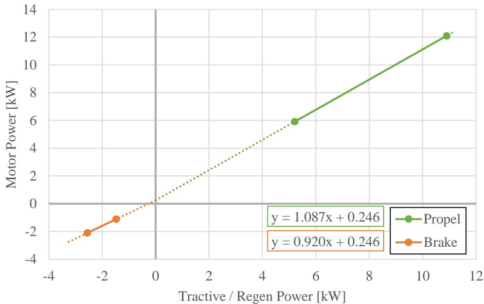
**Figure A.7:** 2021 Mustang Mach-E Extended Range Bi-Directional Willans Line
