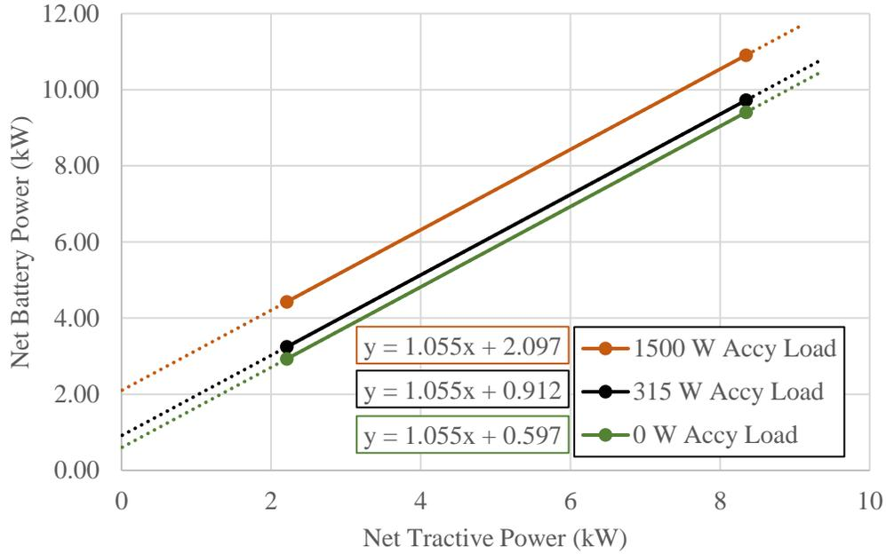
**Figure 4.9:** Model Sensitivity to Vehicle Accessory Load
