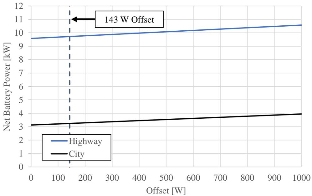
**Figure 4.7:** New Cycle Average Net Battery Power for Specific Offsets
