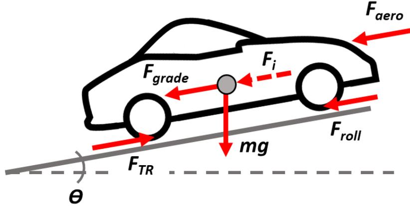
Figure 3.1: Forces Acting on a Vehicle When Driving
