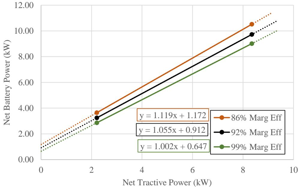
**Figure 4.5: Model Sensitivity to Powertrain Marginal Efficiency**
