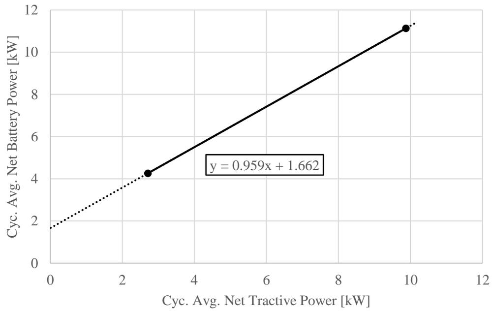
**Figure A.16:** 2019 Tesla Model X Long Range EPA Net Willans Line
