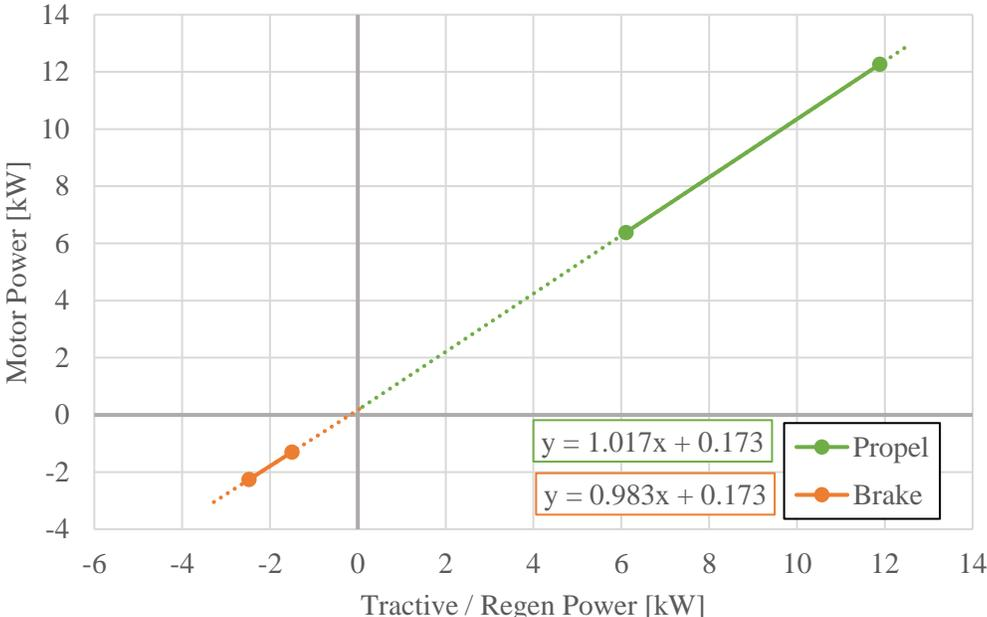
**Figure A.15:** 2019 Tesla Model X Long Range Bi-Directional Willans Line
