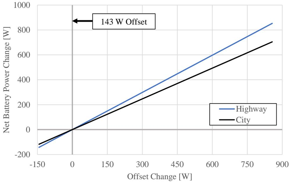
**Figure 4.6:** Net Battery Power Change for Finite Changes in Offset
