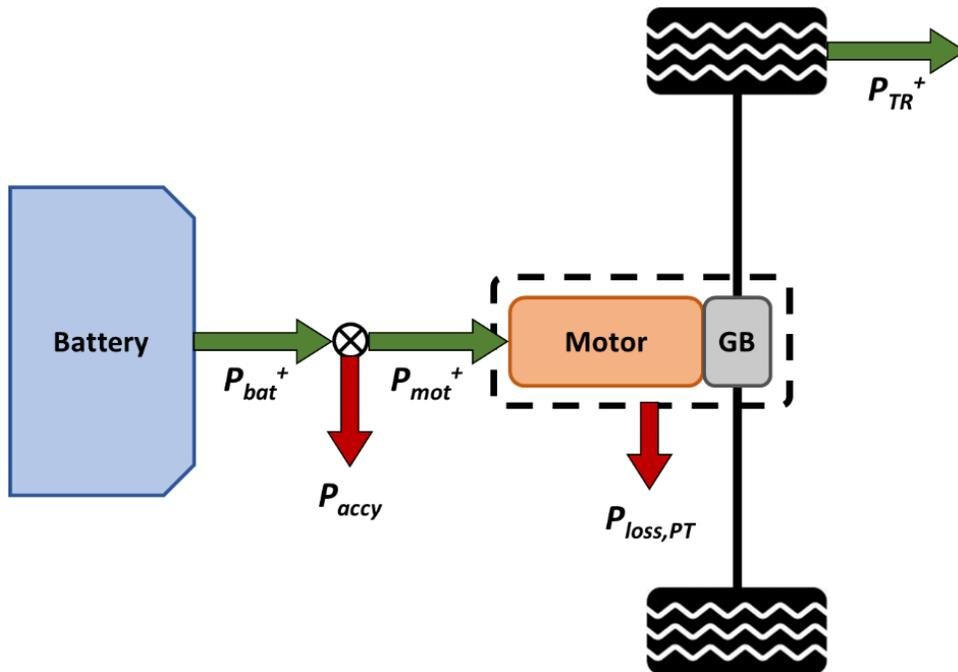
Figure 3.2: Vehicle Propulsion Power Flow
