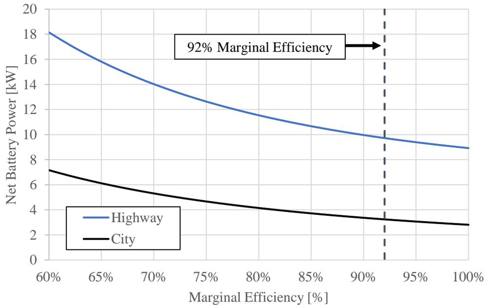
**Figure 4.4:** New Cycle Average Net Battery Power for Specific Marginal Efficiencies
