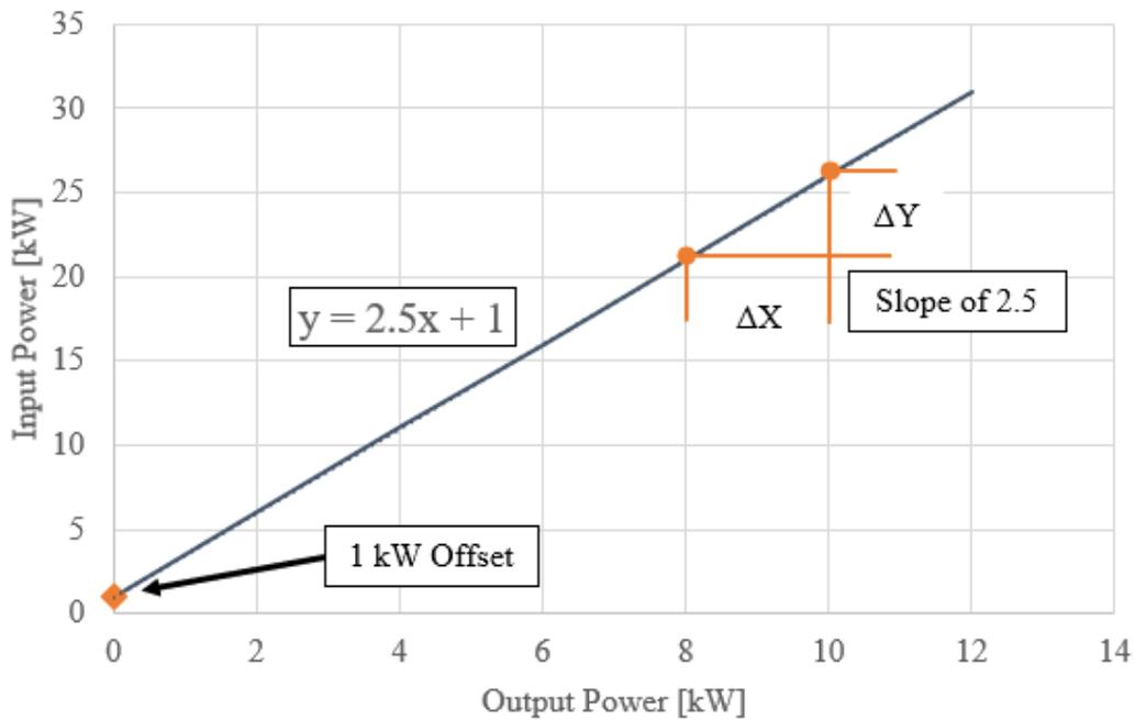
**Figure 1.1:** Willans Line with Labelled Slope and Offset
