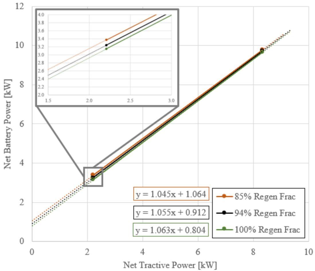
**Figure 4.12:** Model Sensitivity to Vehicle Regen Fraction
