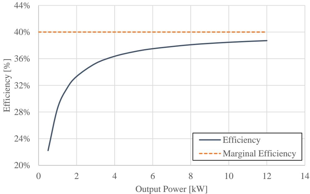
**Figure 1.2:** *Efficiency Curve Derived from Willans Line Slope and Offset*
