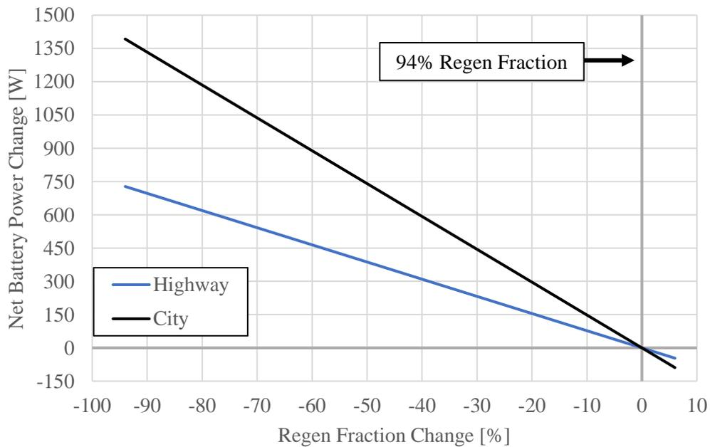
**Figure 4.10:** Net Battery Power Change for Finite Changes in Regen Fraction
