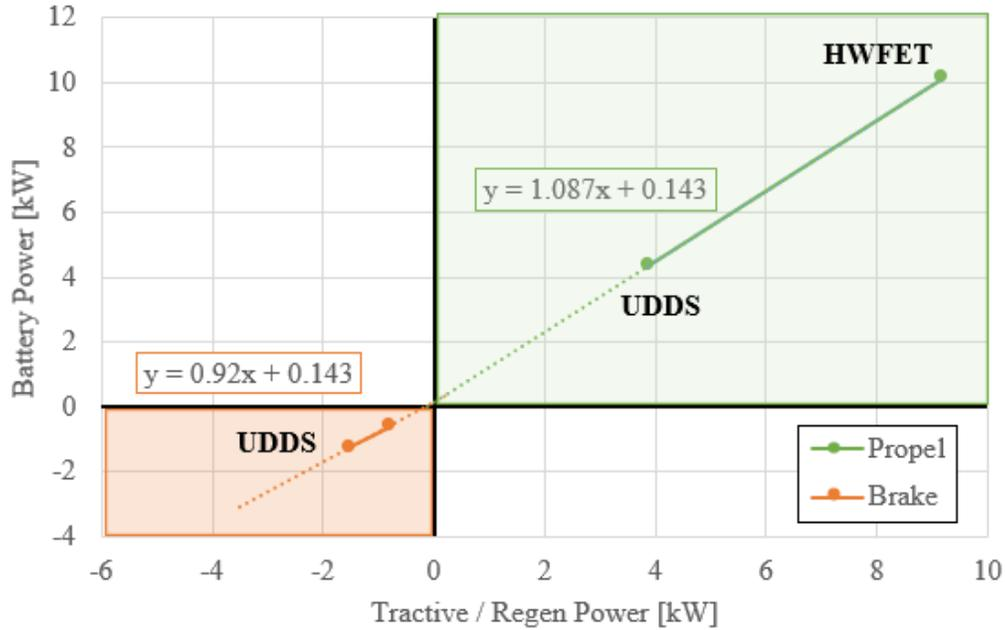
**Figure 3.6:** Instantaneous Battery Power for Propel and Brake Phases
