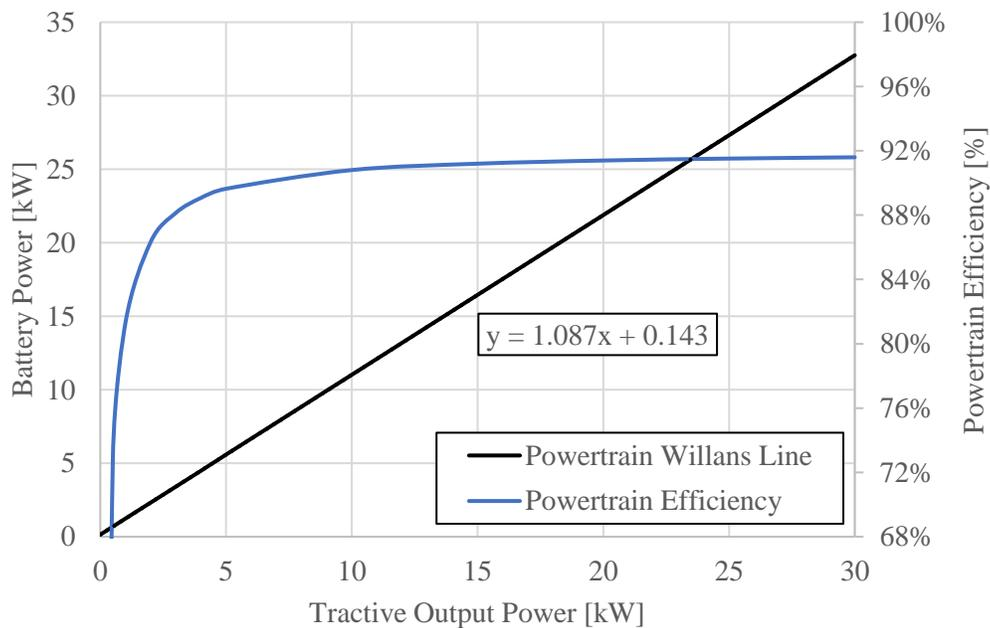
**Figure 4.2:** 2017 BMW i3 Propell Efficiency Curve from Established Parameters
