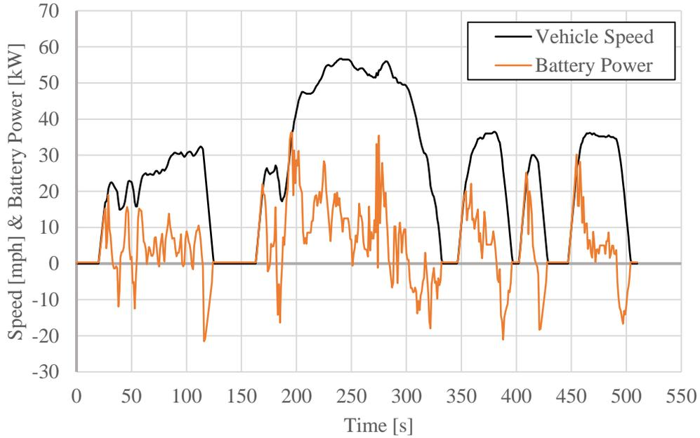
**Figure 3.8:** 505 Speed Profile and Battery Power
