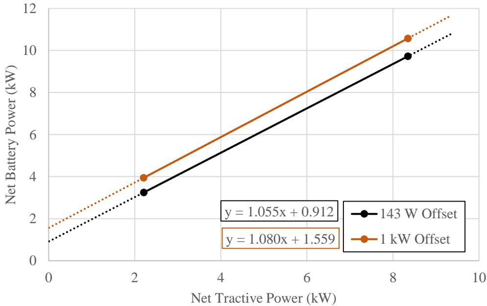
**Figure 4.8: Model Sensitivity to Powertrain Offset**
