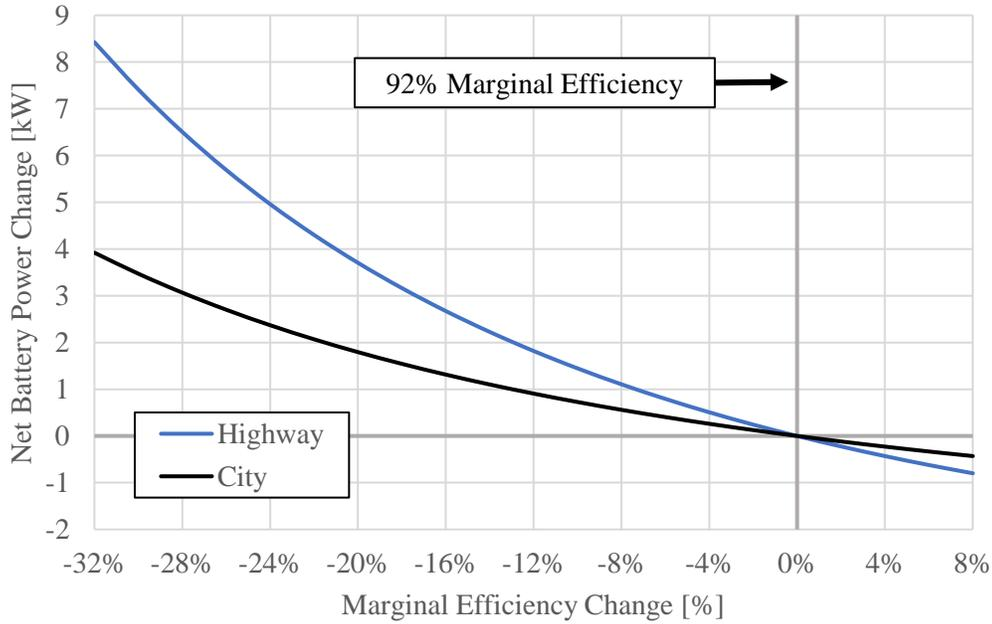
**Figure 4.3:** Net Battery Power Change for Finite Changes in Marginal Efficiency
