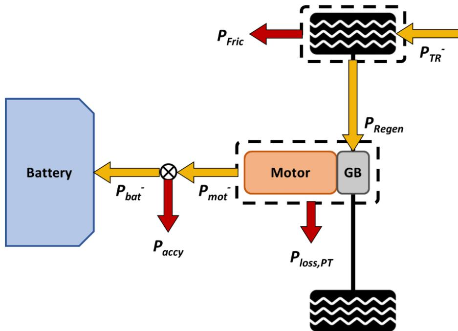
Figure 3.3: Vehicle Braking Power Flow
