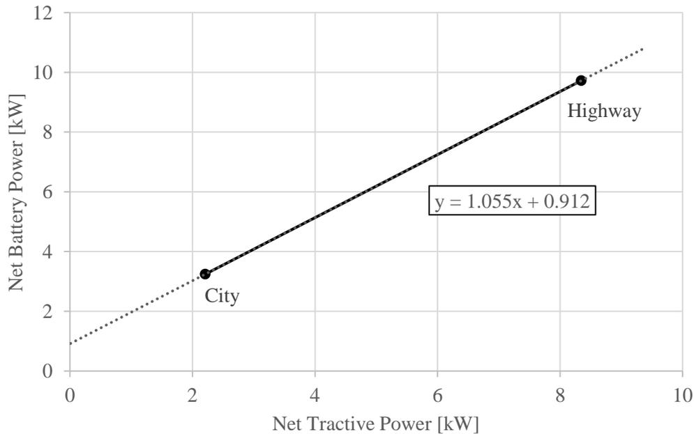
**Figure 4.1: 2017 BMW i3 Derived Net Willans Line Plotted for Two Drive Cycles**
