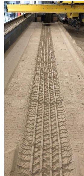
(d) 1 st pass, 12% slip. Ripples are formed.
