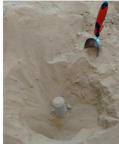
(b) Soil around the sampler was removed by a scoop.
