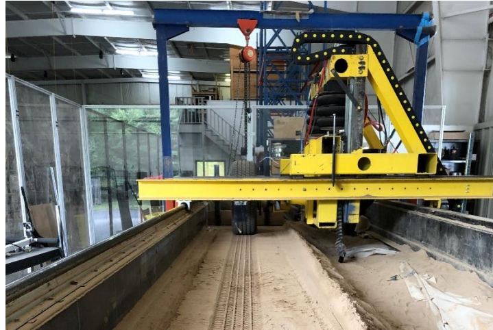
Figure 4.24: Terramechanics Rig in a laboratory free-rolling tire-soil test of 2019.
