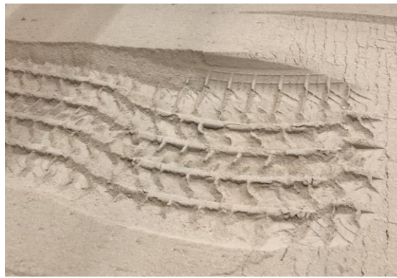
Figure 4.25: Footprint (rut) left by the tire in its final position. The footprint was formed in a static tire-soil test in October of 2019.
