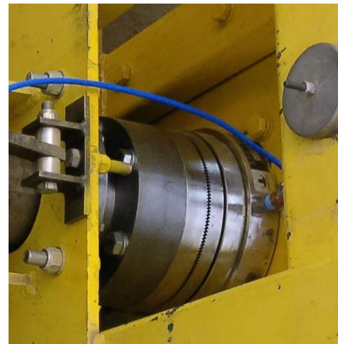
(b) zoom-in view of the clutch.
