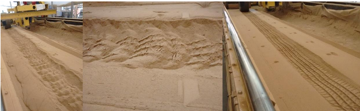
(a) Rut shoulder at the sides of the rut. (b) Rut bottom profile at a high slip ratio. (c) Rut bottom profile at a low slip ratio.
