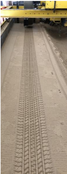
(a) 1 st pass, 8% slip. No ripple is formed.
