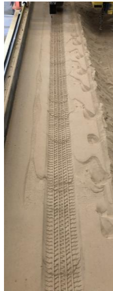
(c) 3 rd pass, 8% slip. More ripples than the 2 nd pass.
