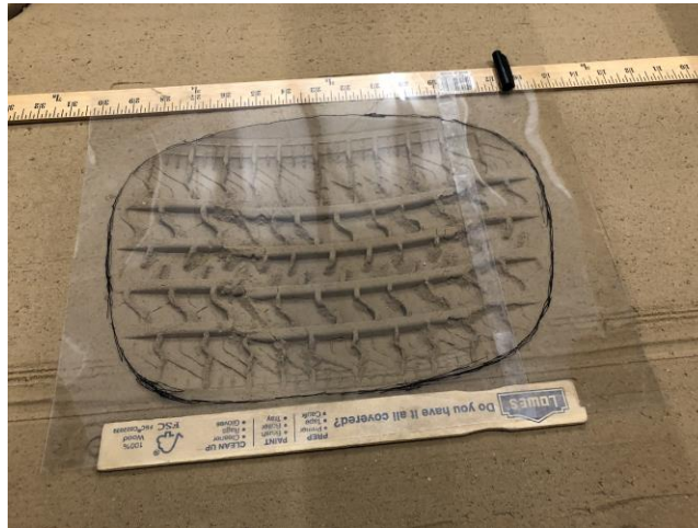
Figure 3.5: Use of two conjunct pieces of plastic sheet to record the rut boundary.
