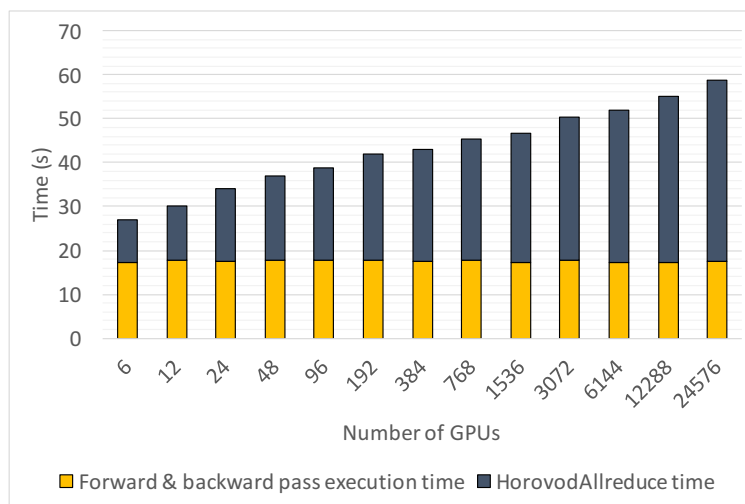
Figure 6.6: TensorFlow/Horovod GPU time breakdown. (We note that using XLA disables any overlap between the computation and communication, as explained in Chapter 6.2.1)
