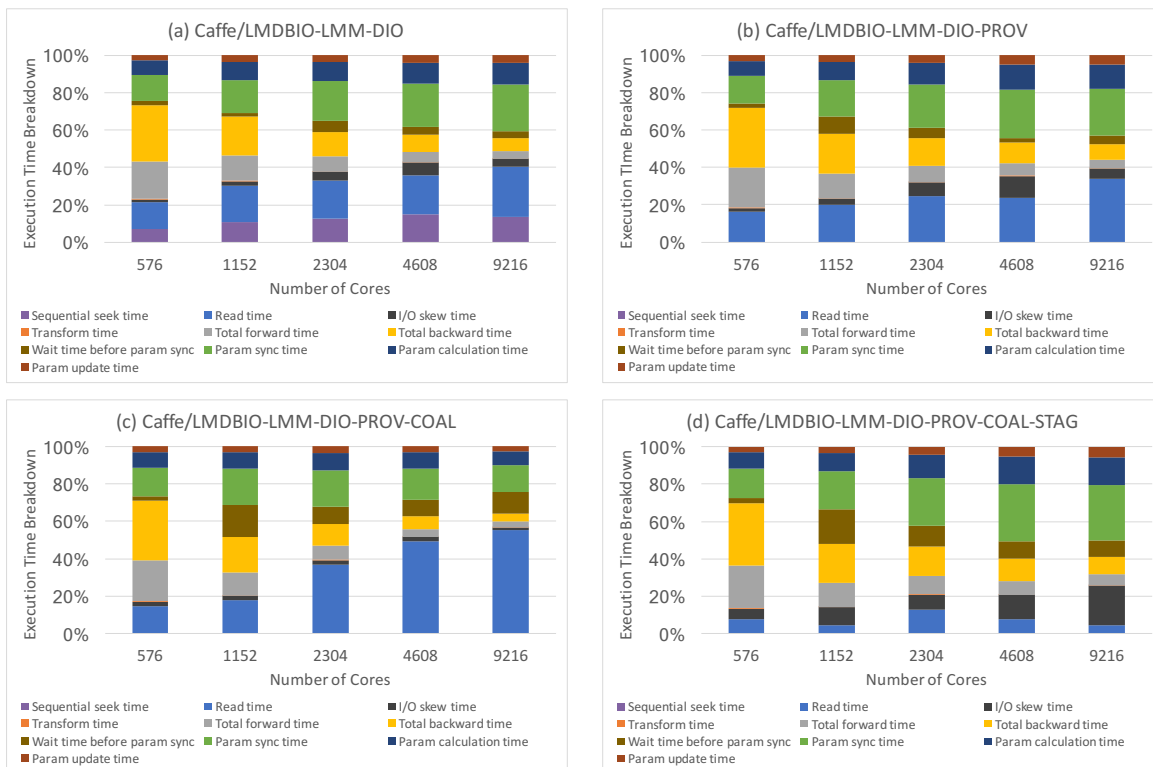
Figure 5.13: Execution time breakdown using ImageNet-Large on Bebop: (a) Caffe/LMDBIO-LMM-DIO; (b) Caffe/LMDBIO-LMM-DIO-PROV; (c) Caffe/LMDBIO-LMM-DIO-PROV-COAL; (d) Caffe/LMDBIO-LMM-DIO-PROV-COAL-STAG
