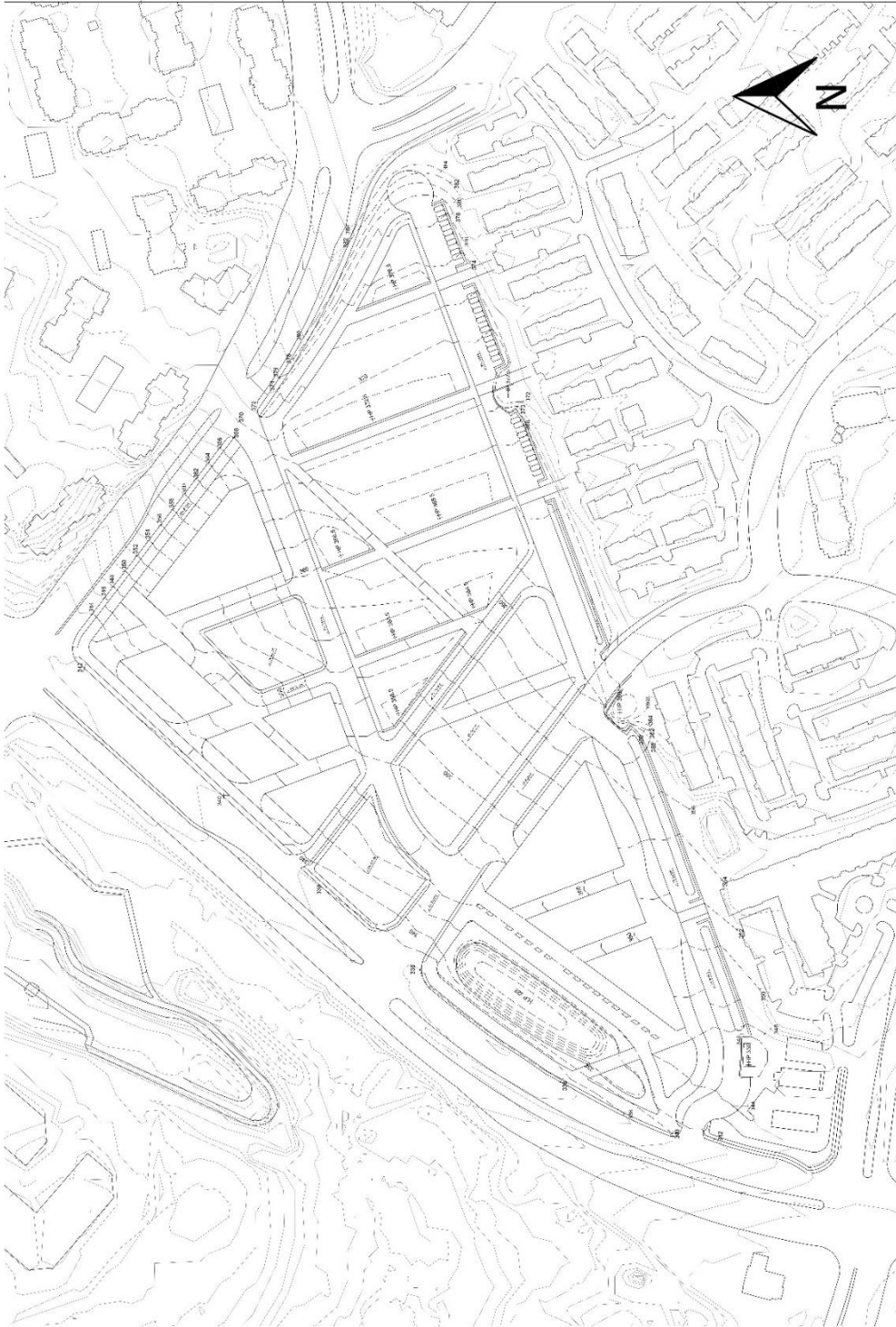
Figure 55: Proposed grading plan, lowest point on the site on bioretention area on the west side.
