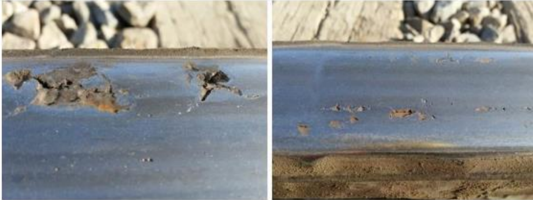
Fig. 1-1. Metal spalling from the rail surface is happened due to rolling contact fatigue.
