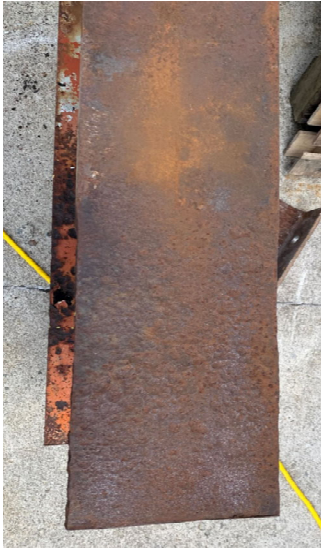
I. Representative Corrosion on the Pre-retrofitted Beam Specimen (BBF Near the End)
