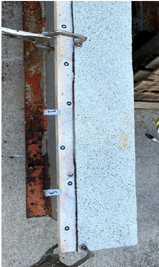
II. Stochastic Pattern on the Pre-retrofitted Beam Specimen (BBF Near the End)
