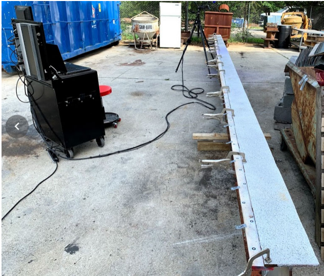
IV. DIC Being Used on the Stochastic Patterned Pre-retrofitted Beam Specimen
