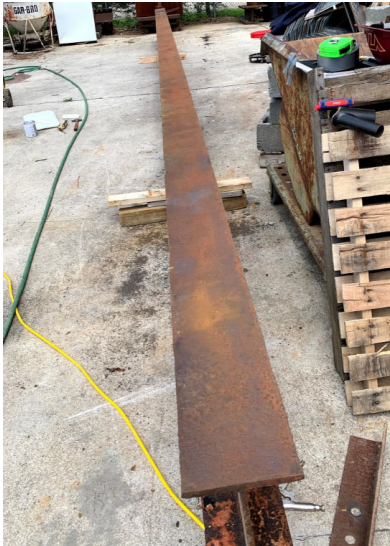
I. Representative Corrosion on the Pre-retrofitted Beam Specimen (BBF Near the End)
