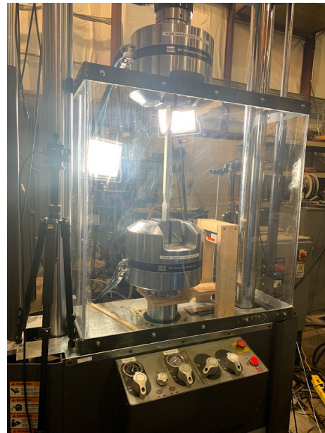
Figure 16. MTS Landmark 370.50 Testing a Double Strap Joint
