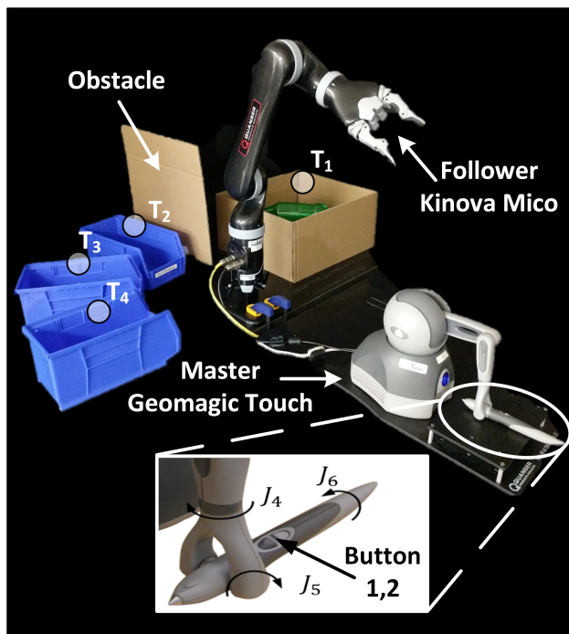
Figure 5.3: Experimental setup with indicated master and follower systems, environmental obstacles, and operational targets (T1-T4).
