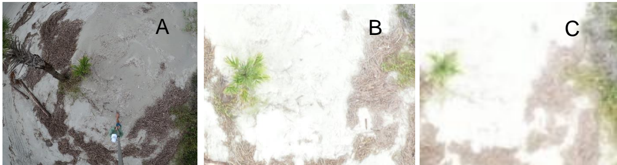
Figure 5: Pole photogrammetry image (A), and 50 m altitude (B) and 110 m altitude (C) drone photos cropped to the same area. Surveys from the pole photogrammetry can produce DSMs and orthophotos of up to 3 mm resolution, while 50 and 110 m drone photos can produce 1.25 cm and 3 cm resolution products, respectively.
