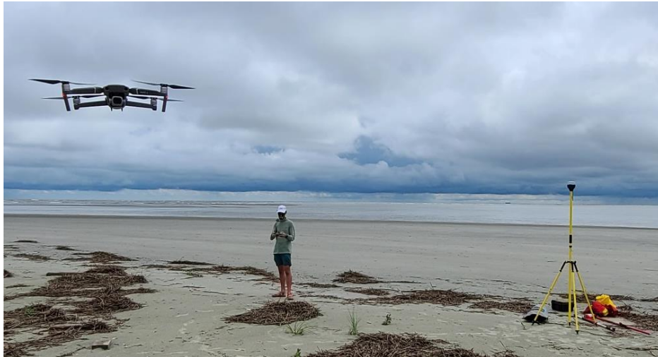
Figure 3: DJI Mavic Pro 2 and Emlid RS2 GNSS base station.
