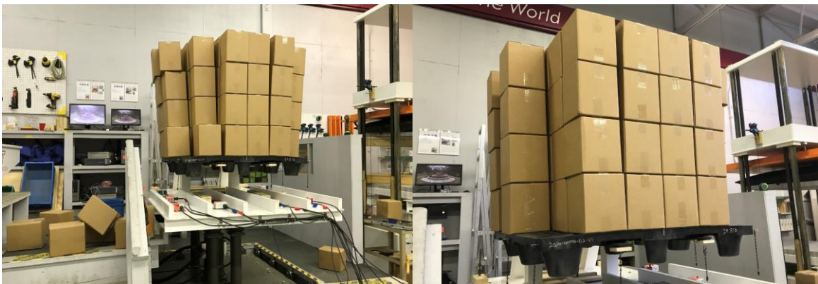
Figure 46. Representative pictures of two of the unbound unit loads after testing.
