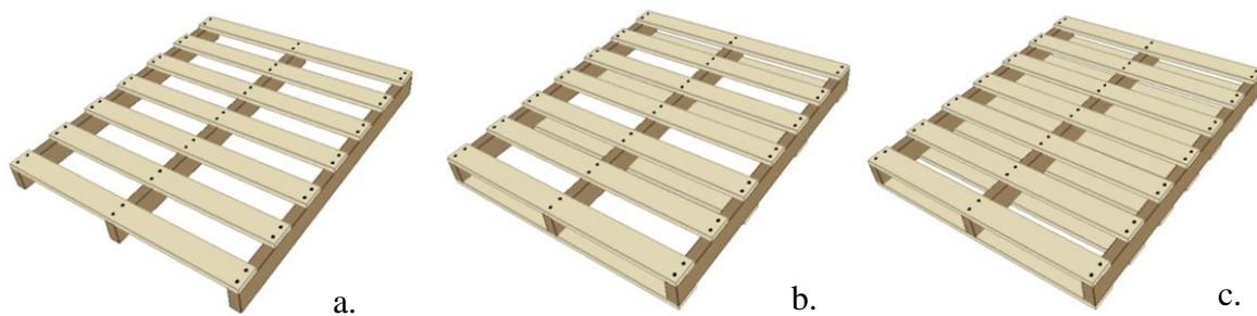
Figure 5. Examples of a) single face, b) double face non-reversible, and c) double face fully reversible pallets
