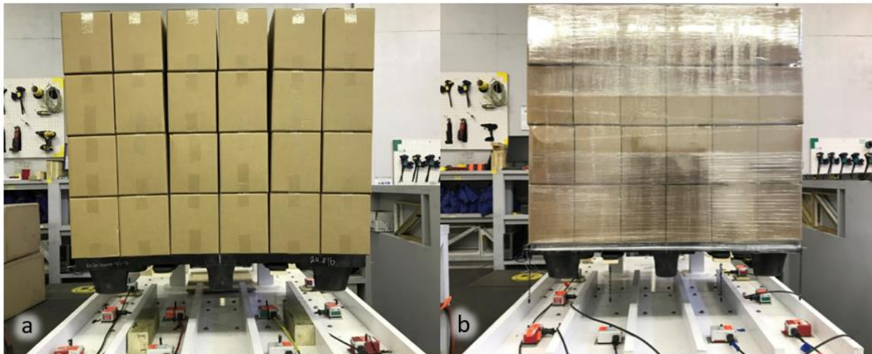
Figure 31. Representative pictures of the unit loads used to conduct the experiments in the across the length orientation: (a) unbounded unit load, (b) bounded unit load
