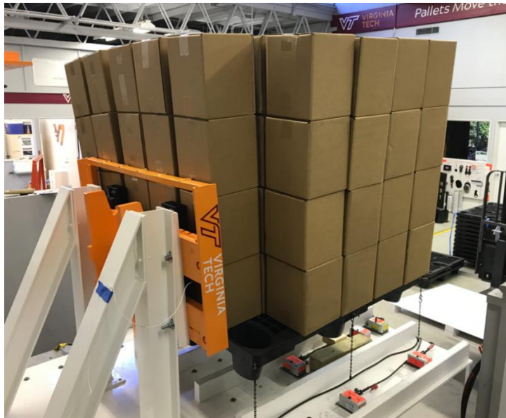
Figure 56. Representative picture of one of the unbound unit loads after the dynamic test in the across the length orientation with initial leveled fork tines.
