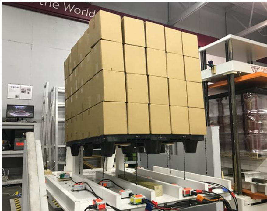
Figure 59. Representative picture of one of the unbound unit loads after the dynamic test in the across the width orientation with initial leveled fork tines.
