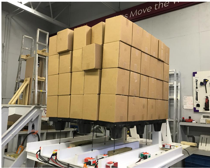
Figure 50. Representative picture of one of the unbound unit loads after the dynamic test in the across the width orientation with initial leveled fork tines.
