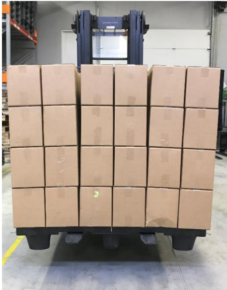
Figure 16. Example of a column stacked unit load supported on a forklift.
