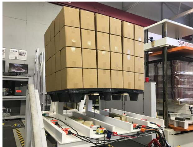
Figure 53. Representative picture of one of the unbound unit loads after the dynamic test in the across the length orientation with initial leveled fork tines.
