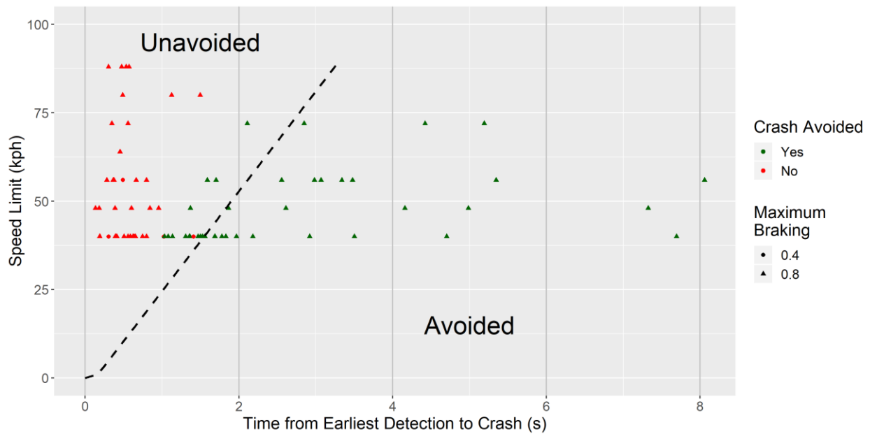
Figure 105. Vehicle speed (speed limit used as surrogate) compared to earliest detection time. The curved line denotes the maximum earliest detection time needed to avoid a crash for a given travel speed. The color of the point indicates whether that cases could be avoided (green) by a system with a 1.5 second TTC of braking and 0 second latency, or not avoided (red).
