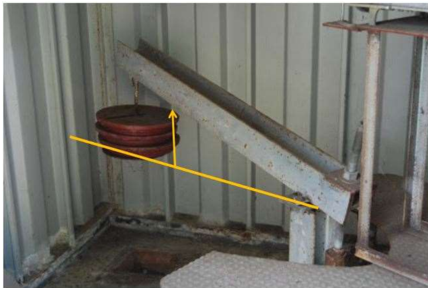
Figure 29. Photographic evidence of land surface rebound with the weighted tensioner of the Franklin extensometer site lifting upwards due to increased tension caused by an increase in distance between the land surface and the bedrock with recovery of previous compaction (David Nelms, personal communication, U.S. Geological Survey, 2019).
