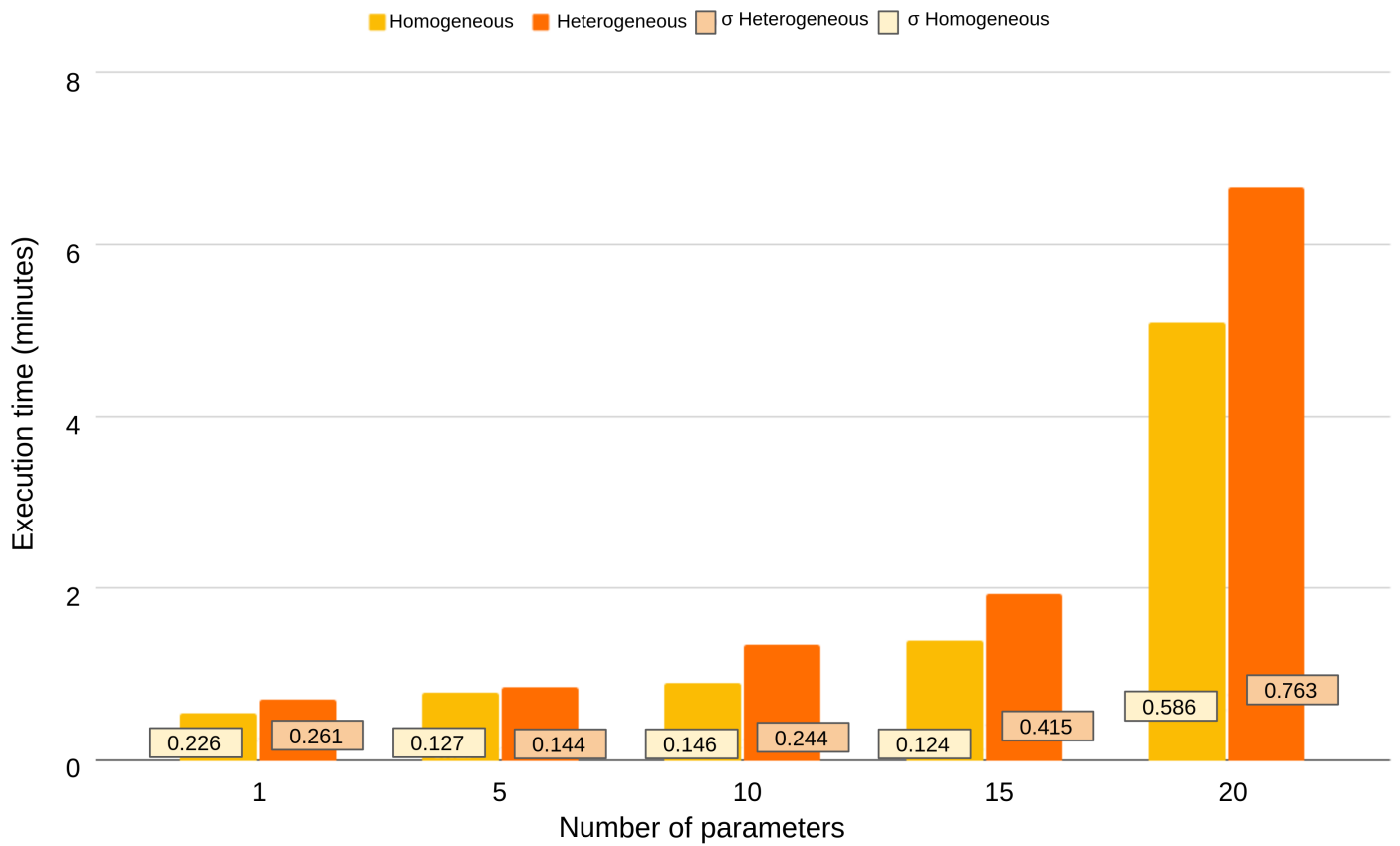
Figure 5.7: Execution of the Parameter-passing overhead microbenchmark for different number of parameters in the enclave functions (from 1 to 20) on homogeneous and heterogeneous setups, and the standard deviations for a 20-runs sample, all of them below one.
