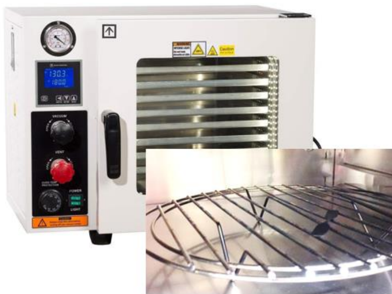
Fig. 3.7: Vacuum Aging Oven for Accelerated Aging
