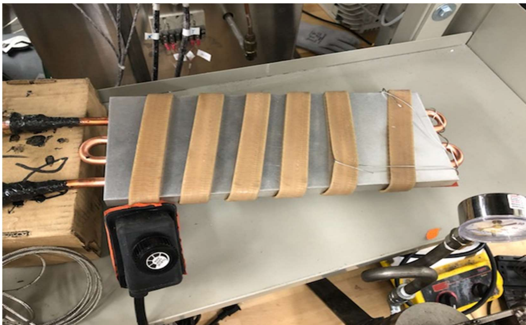
Figure 10: The heat exchanger plate is shown wrapped in electrical heating tape. The heating tape comes with an adjustable thermostat to set the steam or nitrogen temperature used for drying. A thermocouple will be attached to the plate to verify temperature settings.
