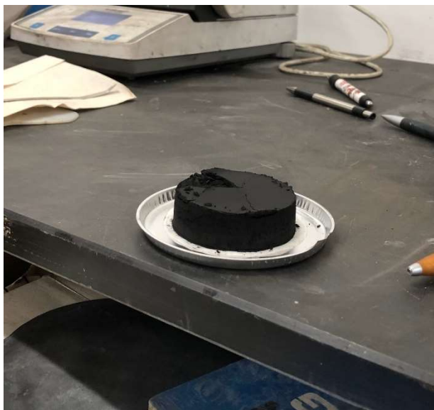
Figure 5: A coal cake removed from the pressure filtration cylinder after the completion of an experiment.
