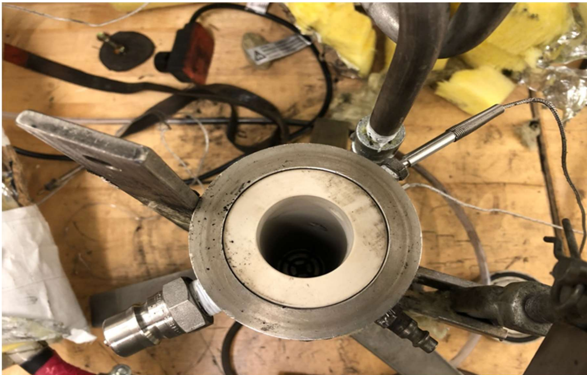
Figure 17: The pressure filtration cylinder with the PEEK insulation tube installed.
