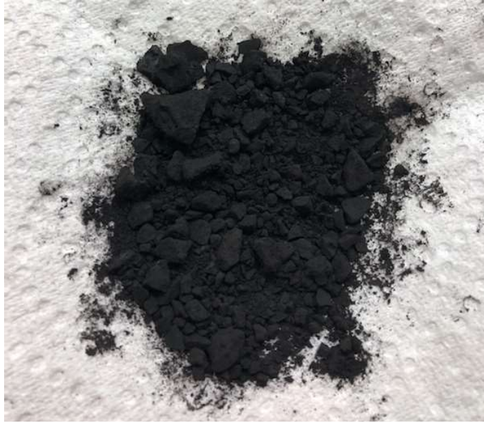
Figure 18: A crumbled coal cake removed from the cylinder after steam drying. There was no condensate visually present on the cake when it was removed. The PEEK insulation tube appeared to solve the steam condensate problem.
