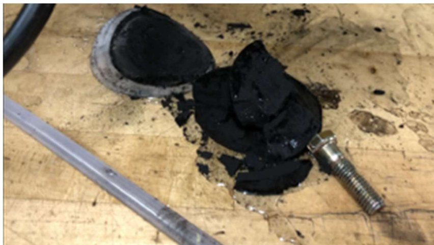
Figure 13: A wet coal filter cake after being removed from the condensate flooded filter. The water on the wood surface around the cake was from steam condensing in the filter cylinder.
