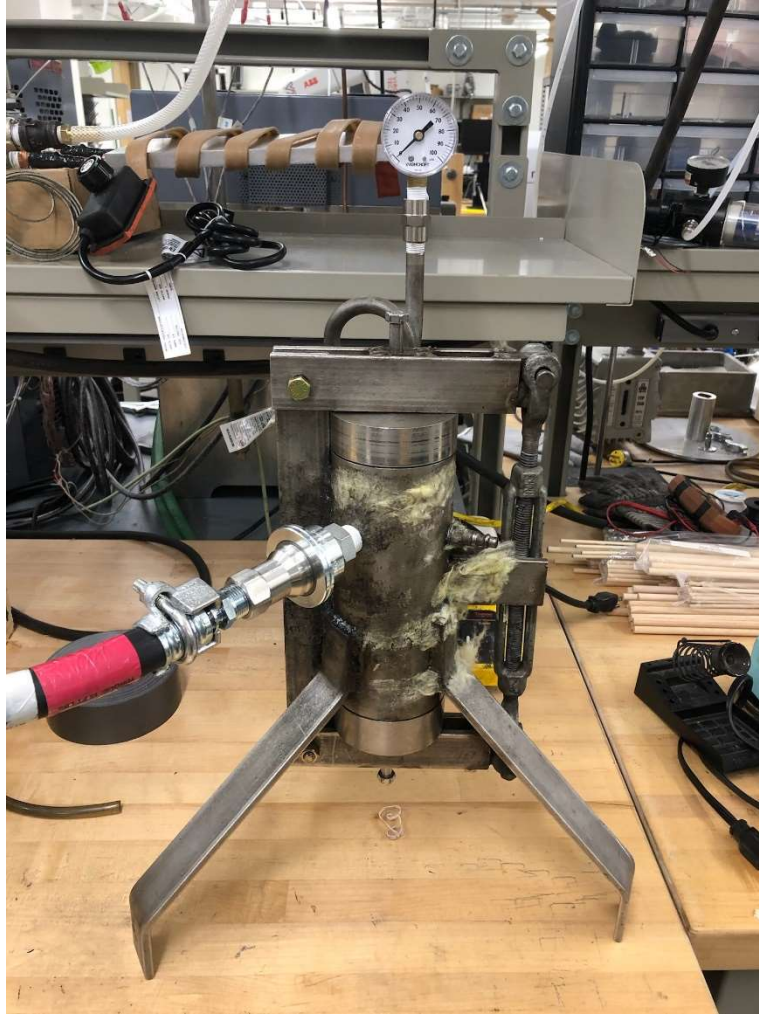
Figure 12: The pressure filtration cylinder modified to accommodate the flexible steam hose for steam injection, and a steam pressure gauge to monitor drying pressure. Insulation was added after taking this photo.
