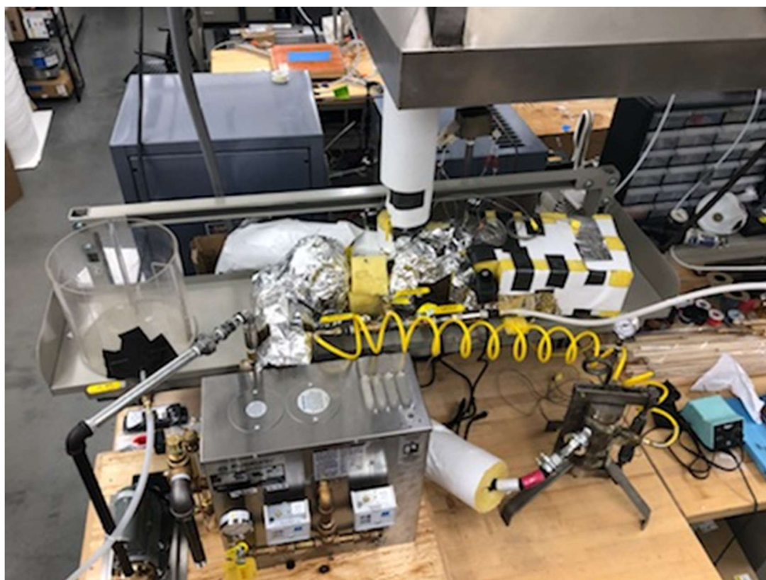
Figure 11: The system is shown with the addition of the 2" thick high temperature fire resistant insulation.
