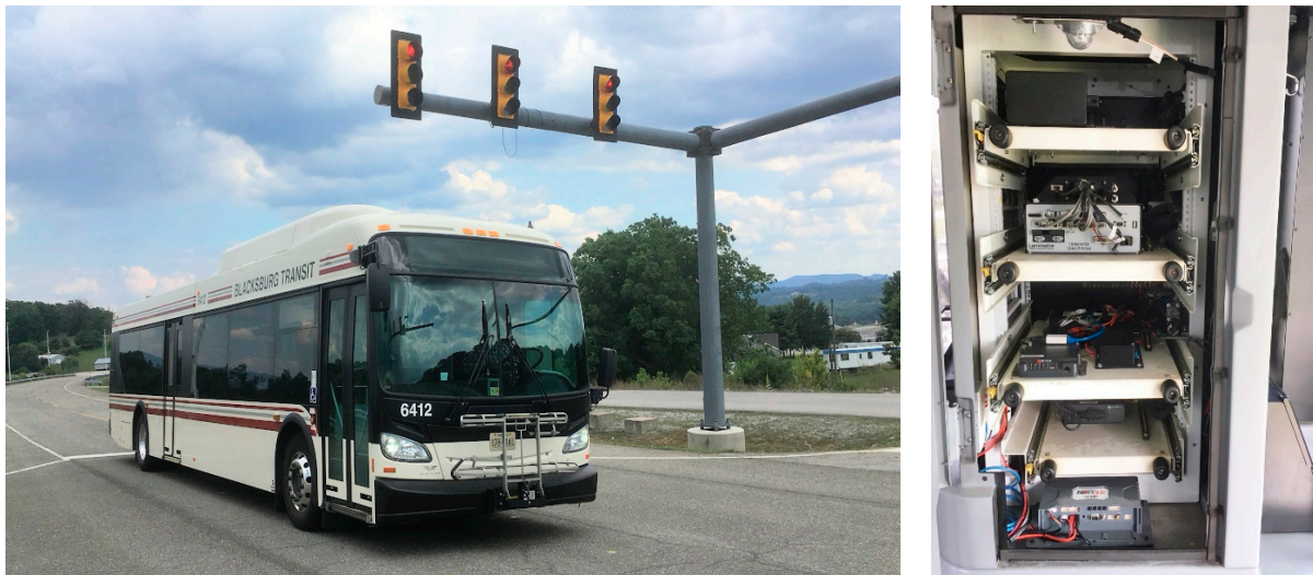
Figure 4. Hardware of the vehicle onboard units in the bus GLOSA system.
