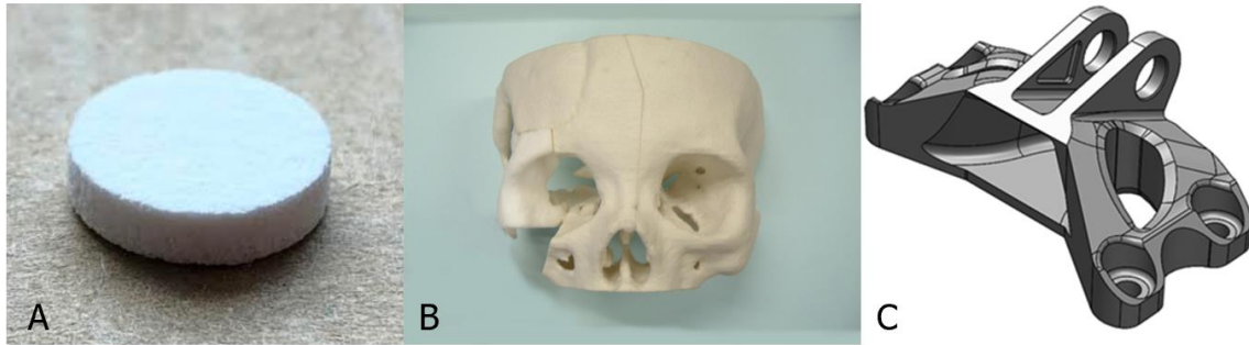
Figure 3.3. BJ AM (A) oral tablets, (B) skull implant for bone replacement, and (C) an engine bracket. (Reproduced with the permission of Wilts et. al. 5 Copyright (2019), American Chemical Society, Patirupanusara et. al. 48 , and Tang et. al. 15 )
