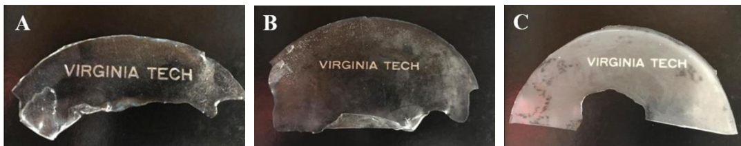
Figure 4.5. (A) Photopolymerized films of TMAEA, (B) TMAEA- co -NVP10 copolymer, and (C) TMAEA- co -NVP30 copolymer.
