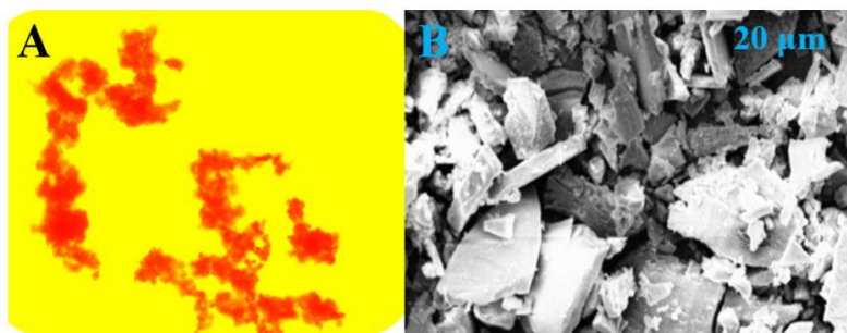
Figure 2.9. EPI-DMA-DIPA and Congo red floc observed using light microscopy (A) and SEM (B). (Adapted from Gupta et. al. 114 )
