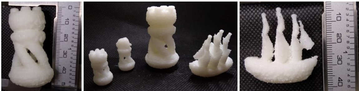
Figure 10.8. PBF printed Spiral Rook 51 (left), ship 52 (right), and part collection (center) using 50:50 powder.
