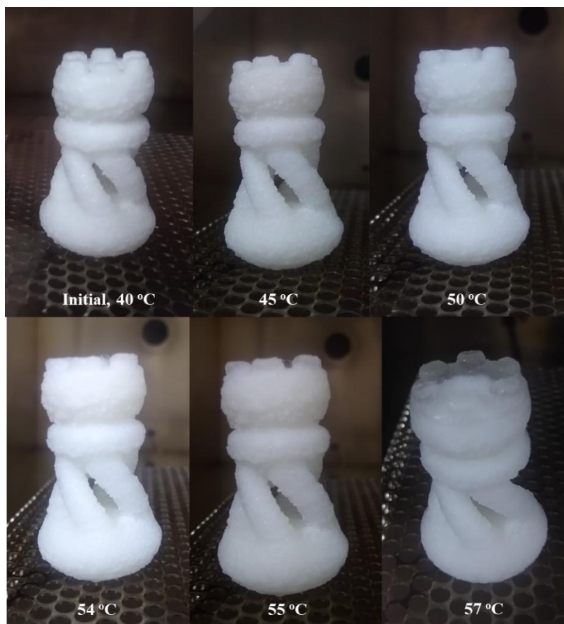
Figure S10.7. Depiction of additively manufactured rook below and above T_m = 51\text{ }^\circ\text{C}
