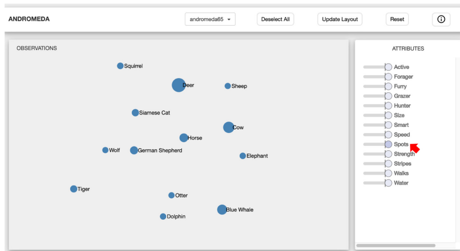
Fig. 5. When hovering on the Spots slider, the radius of each data point changes in proportion to its Spots values.
