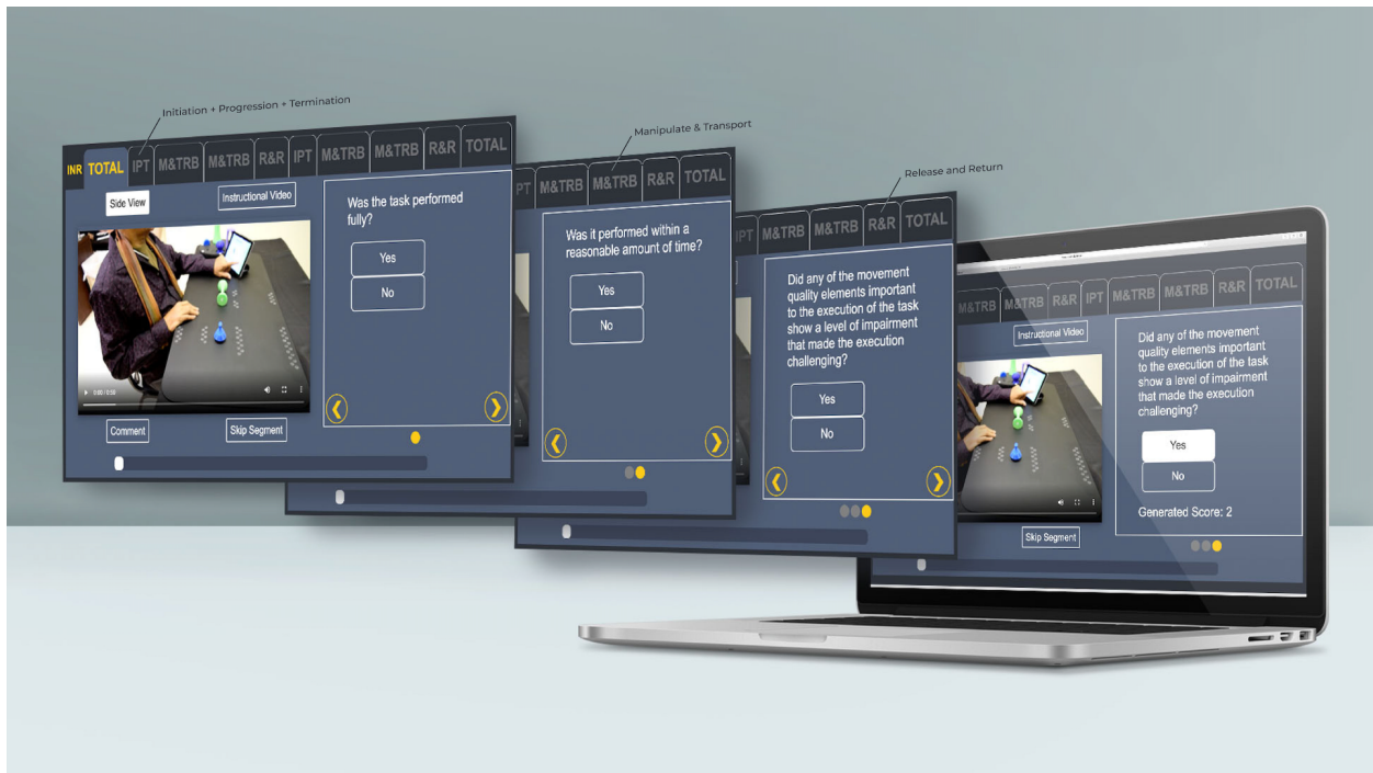
Figure 4.4: The video annotation tool presents the therapist with both sagittal- and front-captured videos of the stroke survivors/patients attempting one of the 12 ADL tasks, in addition to an instruction video of an unimpaired person doing that particular ADL, which the patients had viewed before attempting the task. The goal of the tool is to assist the therapist in evaluating the quality of the patient movement performance.
