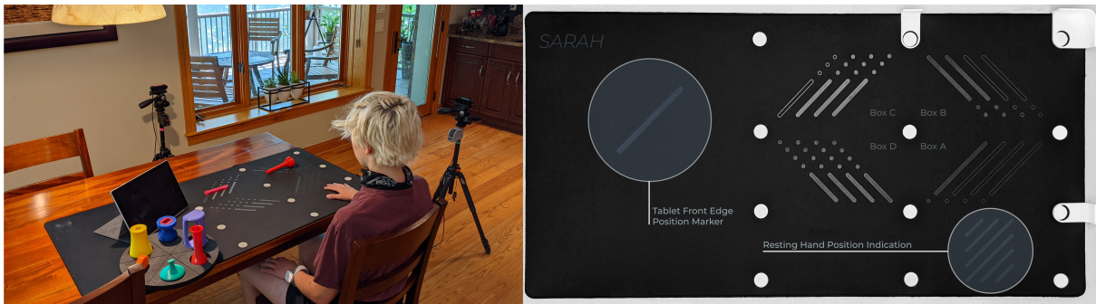
Figure 4.2: The Sarah System is an in-home based rehabilitation system which consists of a two-camera setup, tablet interface, a customizable activity space, and 3D-printed objects
