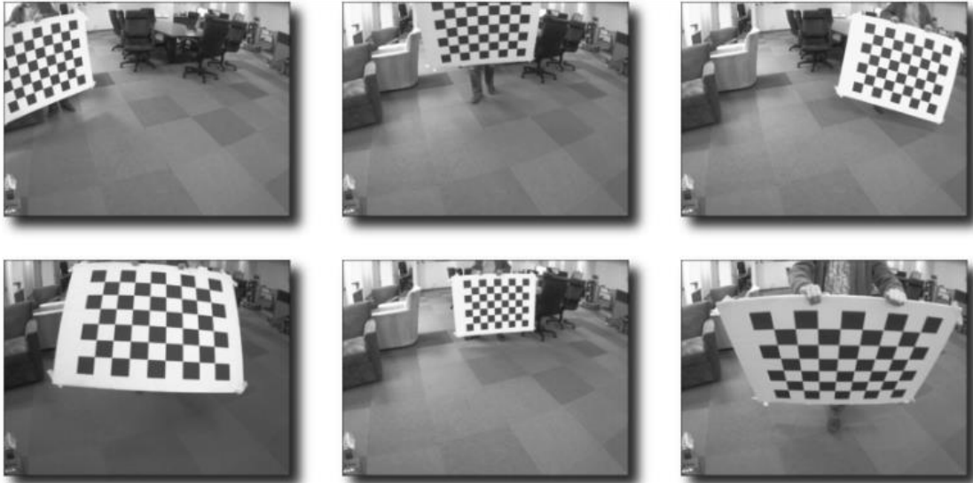
Figure 4: Example of moving the checkerboard around the camera field of view.
