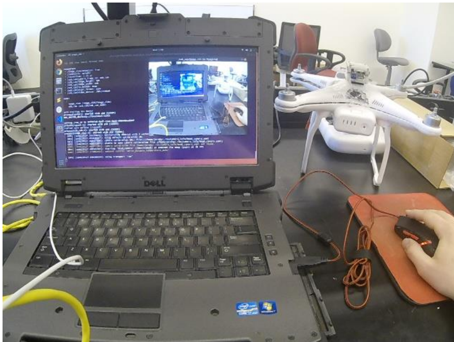
Figure 8: Running usb_cam and image_view to view camera output
