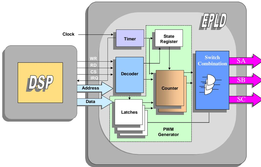
Figure C-2. EPLD functional block diagram for the three-phase VSI
