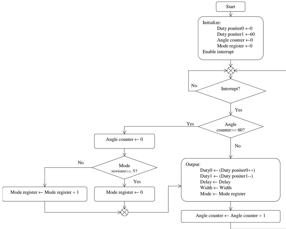
Figure C-3. Flow diagram of the DSP program
