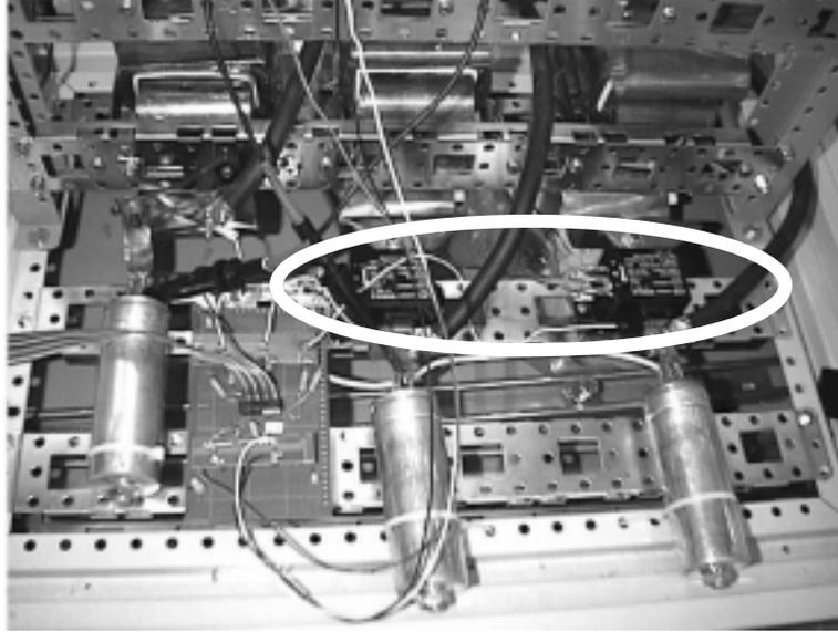
Figure C-5. Current sensors placed after main inductors
