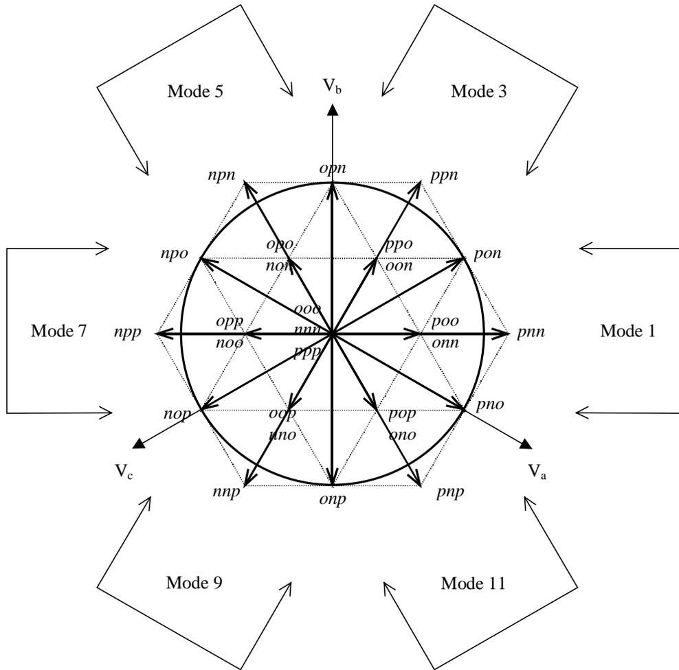
Figure C-1. Space-vector representation and its mode assignment of the three-level VSI
