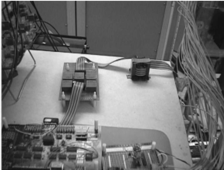
Figure C-6. Voltage sensors and CM choke for three AC outputs and two DC inputs
