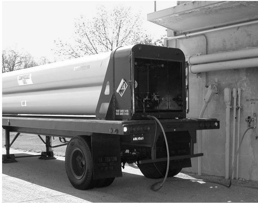
Figure 2.7: Tuber truck supplying high-pressure air for the TEB flow control system.
