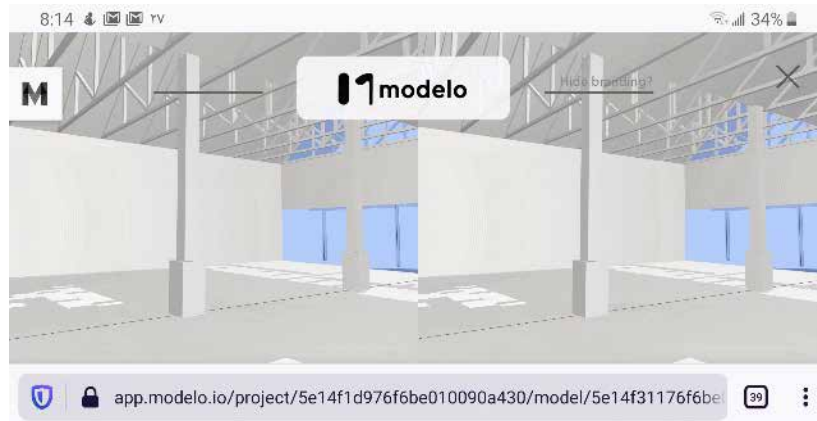
Figure 6-13 A screenshot from the video demonstrating interior study of the design using VR through Modelo
