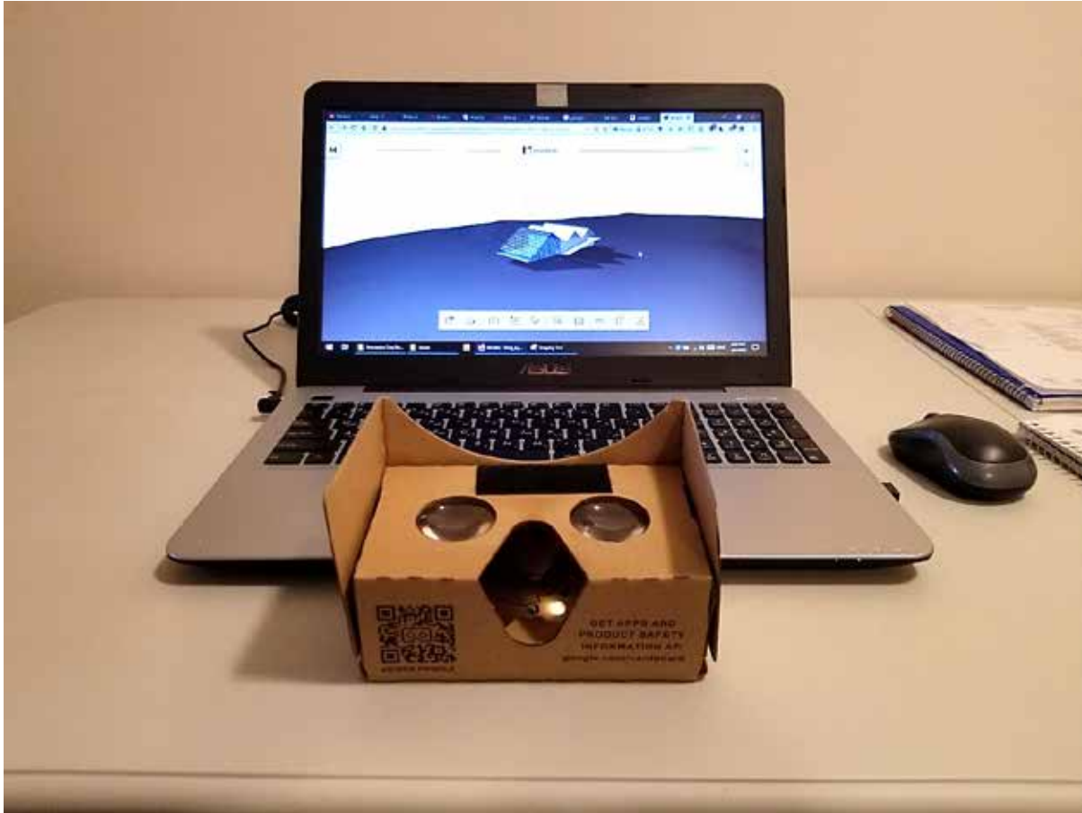
Figure 7-18 Using Modelo and Google Cardboard to incorporate VR for interior studies
