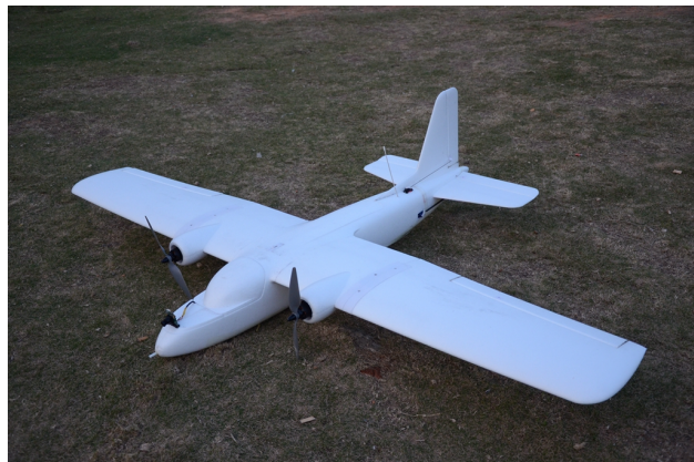
Figure 4.1: My Twin Dream fixed-wing experimental aircraft used at the Nonlinear Systems Laboratory (NSL) at Virginia Tech [23]
