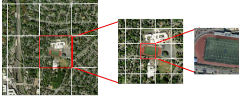
Figure 6: A demonstration of how each zoom level works in the context of raster images.
