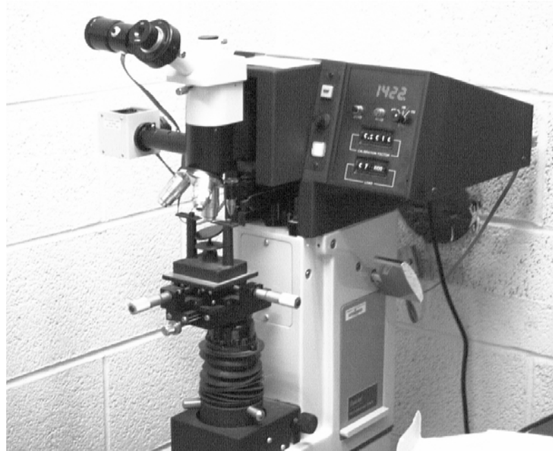
Figure 2.9. Vickers indentation tester, Tukon 300, Instron Inc.
