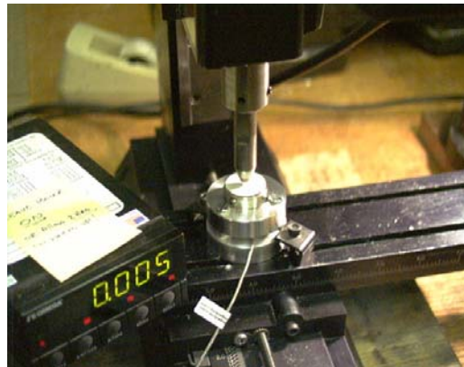
Figure 2.6. Ball on ring test fixture.
