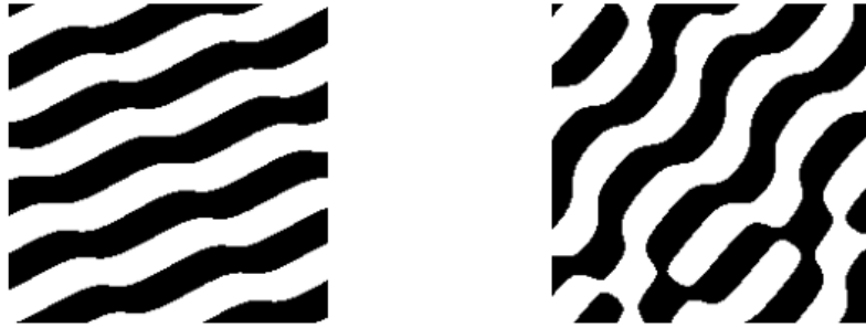
Figure 4.1: The two spinodoids and their \theta values that are solutions to the first inverse design problem of targeting a specific Young's modulus of 1.636 GPa. Figure derived from [60].
