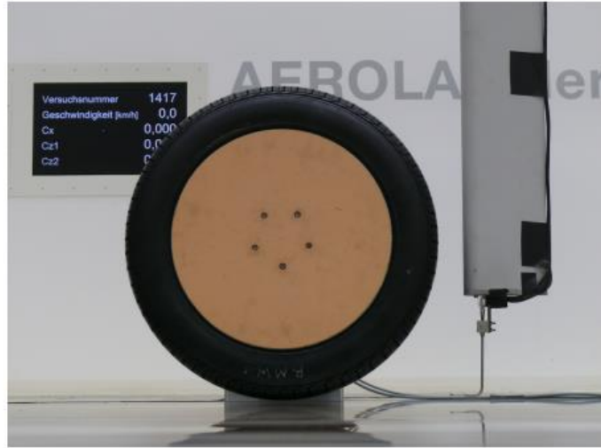
Figure 1-5: Tire Experimental Setup with Probes [25]
