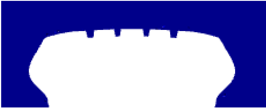
Figure 4-16: Tire Cross Sectional Profile for the Highest Drag Case
