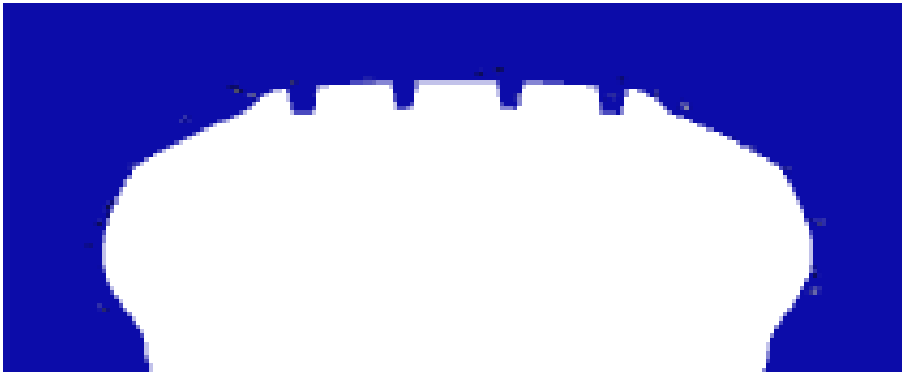
Figure 4-15: Tire Cross Sectional Profile for the Lowest Drag Case
