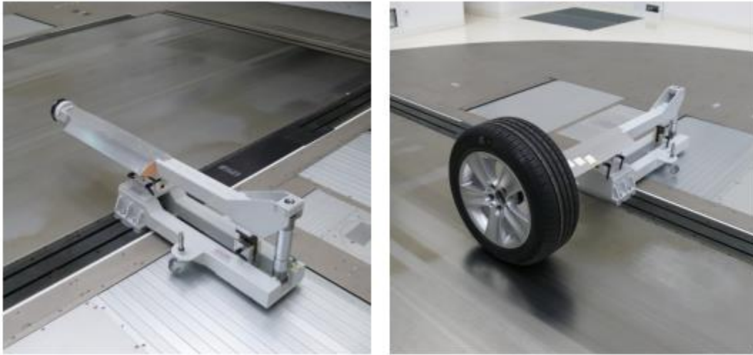
Figure 1-4: Standalone Tire Experimental Setup [25]
